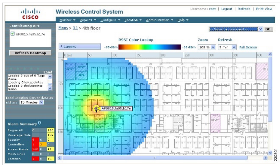
Figure 8.1: Example of access point placed onto a floor map in Cisco Prime [27].
