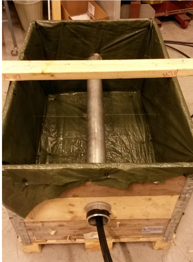
Figure 6.2: Tarpaulins were installed inside all models. The picture was taken before installing thermocouple probes.
