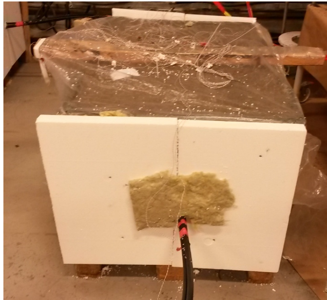
Figure 6.9: One of the models after installing styrofoam and rockwool.
