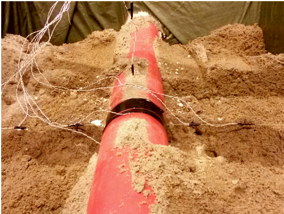
Figure 6.8: Assembling the probes by the help of fireline.
