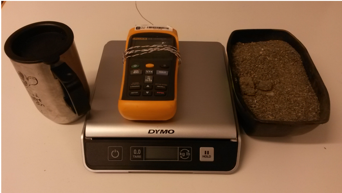
Figure 7.2: Equipment used for measuring the specific heat capacity in the sand.
