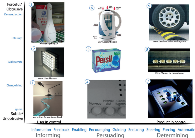
Figure 3: The obtrusiveness-control landscape. A two dimensional landscape of design strategies created by the axis of Obtrusiveness and distribution of control. Illustrated with 9 examples of strategies with variations of both dimensions.
