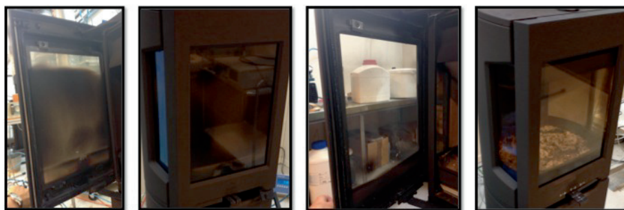
Figure 4.31. Soot on glass door after the testing. The conventional woodstove to the left and the prototype to the right.
