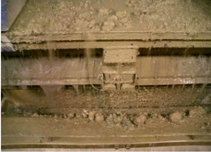
Figure 30: Sticky cuttings coming over the shaker (Christophersen et al., 2007).
