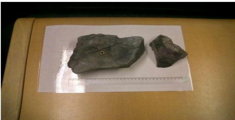
Figure 31: Cuttings found in bell nipple during clean up(Christophersen, Gjerde, & Valdem, 2007).
