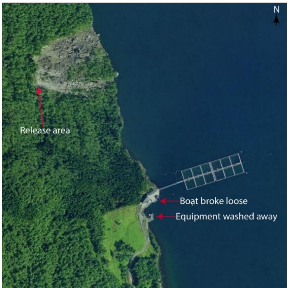
Figure 1.5: Orthophoto showing the northeast sector of the unstable area. The fish farm is located approximately 450 meters south of the impact area. Location of the boat that broke loose and the damaged equipment are indicated. Length of the fish farm is 240 meters. Modified from Kartverket (2015).
