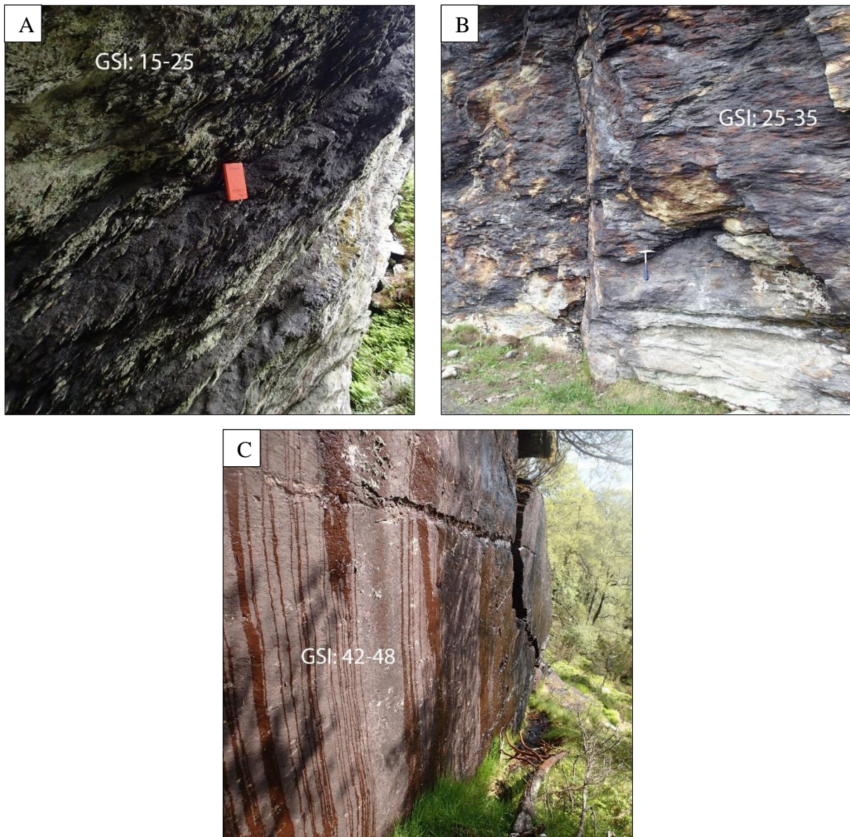
Figure 4.23: Examples of outcrops where GSI was estimated. A: Outcrop close to location 16 with graphite. GSI range: 15-25 B: Outcrop at location 1 showing weathered phyllites with a GSI range of 25-35 C: Outcrop south of location 30. GSI range: 42-48.
