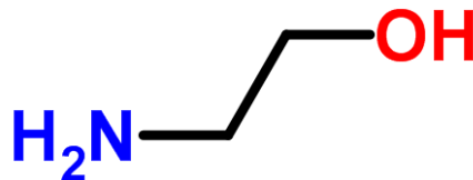
Figure 2.3 Molecule structure of monoethanolamine (MEA)
