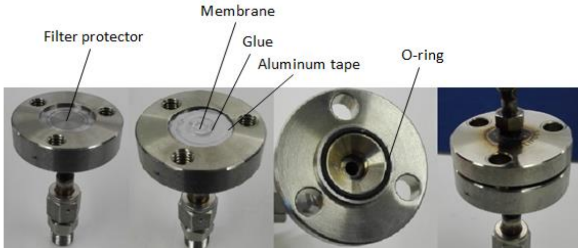
Figure 17. Montage of the membrane in the module.
