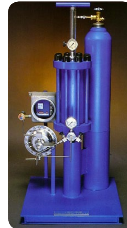
Welker light liquid hydrocarbon sampler.
