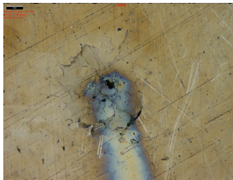
Figure F.6: Surface characterization of pit on sample 2.29 by 3D OM after anodic CPP, with a magnification of 20X.
