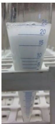
Figure 39: Bottle test tube containing a filtrated surfactant-stabilized o/w model oil emulsion, filtrated through filter no. 4. No free oil formed in the bottle test tubes immediately after filtration, but a foam layer containing larger droplets was observed.
