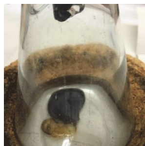
Figure 27: Free water formed in the filtration flask during filtration of the 50:50 wt. % Crude Oil A and B mixture emulsions.
