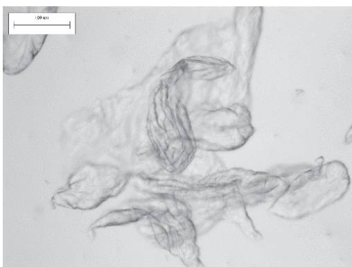
Figure 45: Microscope image of the gel formed on top of the filter when filtration of particle-stabilized o/w model oil emulsions of hexadecane and water, containing 30 vol. % oil cut, stabilized with 0.5 wt. % Aerosil R7200, emulsified at 24000 rpm for two minutes. No existing droplets can be seen. Magnification 10x. Size mark: 100 \mu\text{m} .
