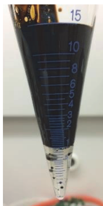
Figure 20: Bottle test tube containing a filtrated Crude Oil A emulsion. Free water was formed after filtration through filter with porosity number 3. Parallel 2
