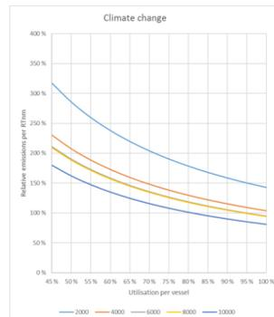
For all analysis, an emission level of 100% was assumed for the 6000 RT vessel at 95% utilisation. The figure on the left shows that the lowest environmental impact is obtained by the 10,000 RT vessel, and the highest impacts are related to the 2000 RT vessel.
