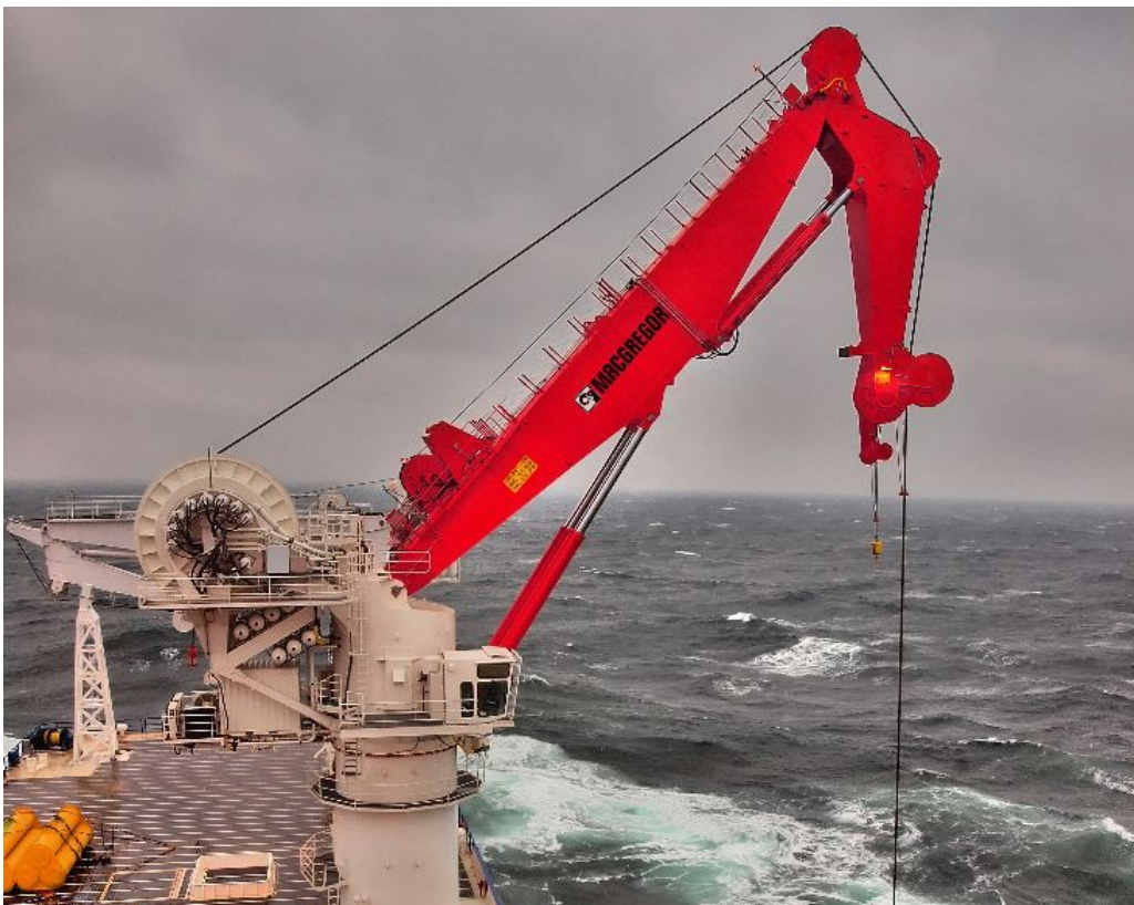
Figure 5.1: Considering the fact that MacGregor's AHC offshore crane is placed on board a ship the environment is of concern. Reproduced with kind permission from MacGregor.
