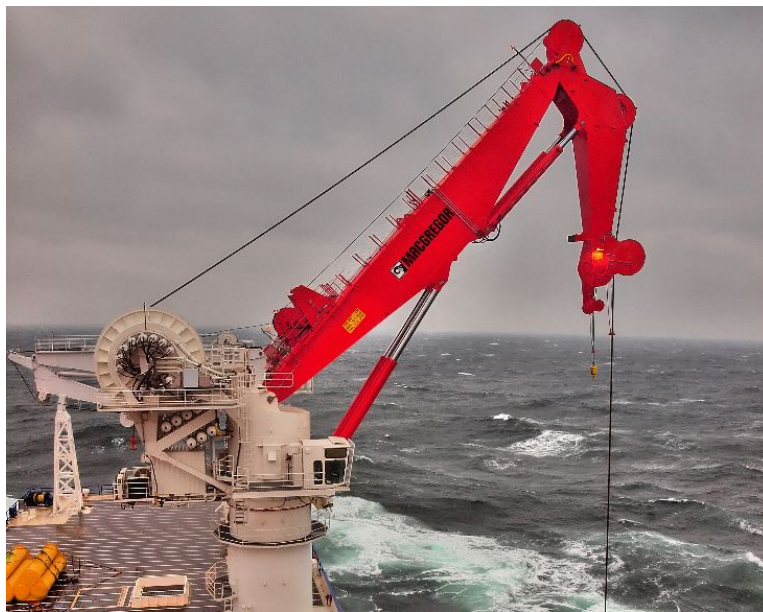
Figure 1.1: MacGregor's AHC offshore crane operating under rough weather conditions. Reproduced with kind permission from MacGregor.
