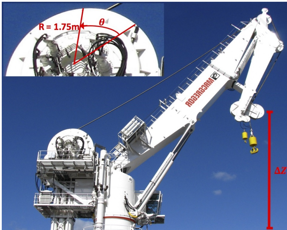
Figure 4.3: Illustrating the dynamics of the wire compensating with a constant radius of 1.75 m. The drum will initiate the opposite movement of the influence of the waves upon heave.
