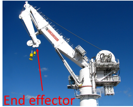
Figure 2.2: MacGregor's crane with it's end effector labeled. Reproduced with kind permission from Mac-Gregor.
