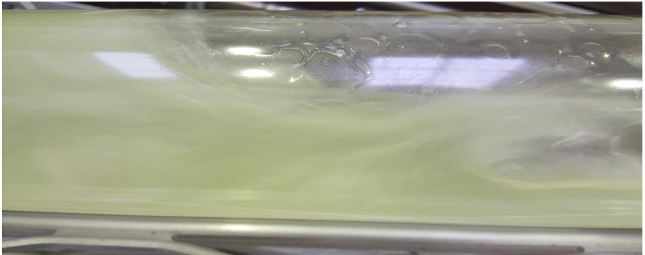
Appendix Figure 5. Churn Flow (AIR-WATER) (15 degrees inclination, U_{sl} = 1.1 m/s, U_{sg} = 0.82 m/s)
