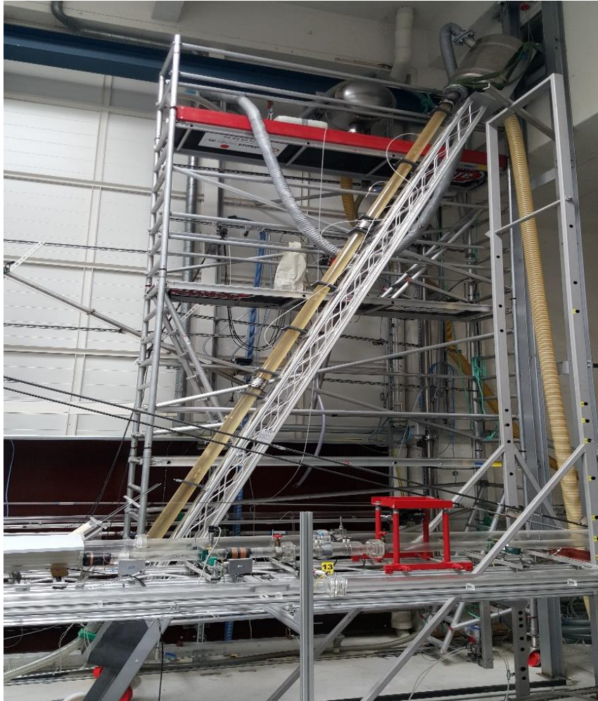
Figure 2.11. The inclinable test rig with the annulus test section in operation
