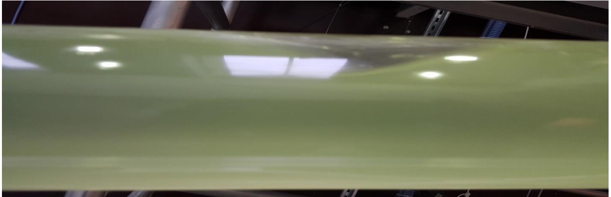
Appendix Figure 3. Bubble Flow (AIR-WATER) (15 degrees inclination, U_{sl} = 0.96 m/s, U_{sg} = 0.17 m/s)
