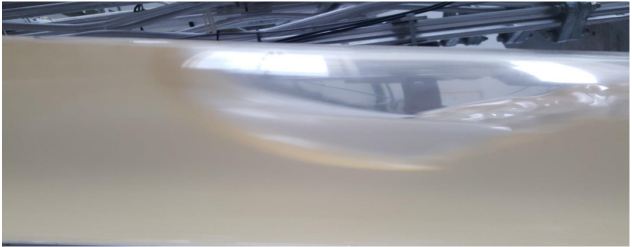
Appendix Figure 7. Bubble Flow (AIR-OIL) (15 degrees inclination, U_{sl} = 0.58 m/s, U_{sg} = 0.11 m/s)
