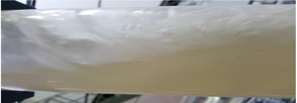
Appendix Figure 9. Churn Flow (AIR-OIL) (15 degrees inclination, U_{sl} = 0.96 m/s, U_{sg} = 0.78 m/s)
