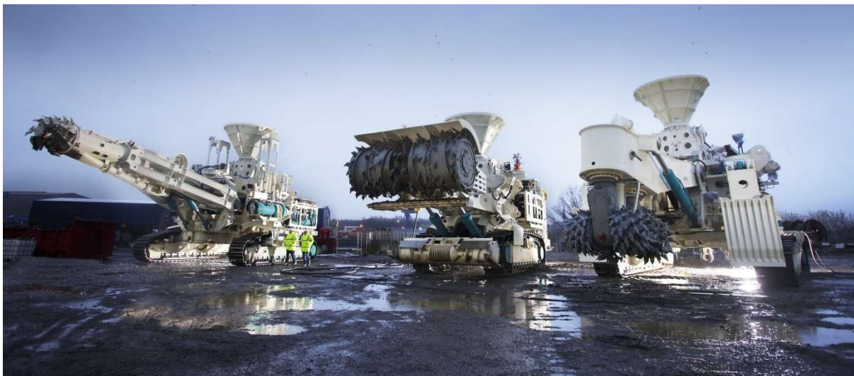
Figure 3-30 – From left: Collecting machine; bulk cutter; and auxiliary cutter (Nautilus Minerals) 8 .
