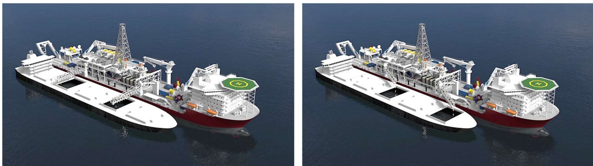
Figure 3-43 – Side-by-side offshore loading of bulk carrier (Nautilus Minerals 9 ).
