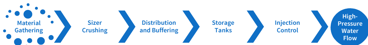
Figure 3-23 – Functionalities of Technip’s Subsea Crushing and Feeding Unit (SCFU).
