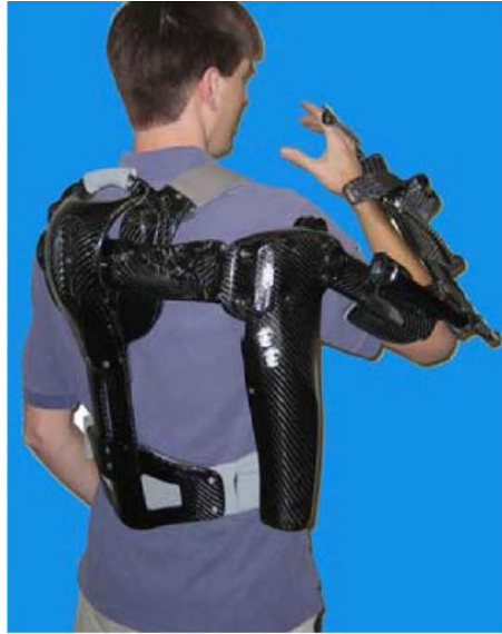
Figure 2.2: RUPERT - Exoskeleton Robot, picture taken from [32]
