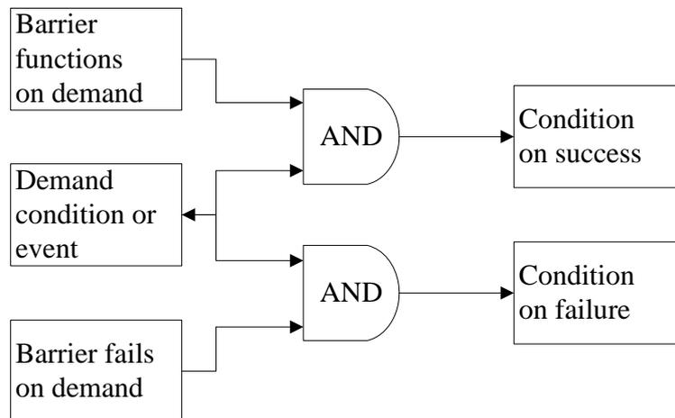
Figure 6: Representation of the barrier from Figure 5 by means of a FT (from Duijm, 2009).
