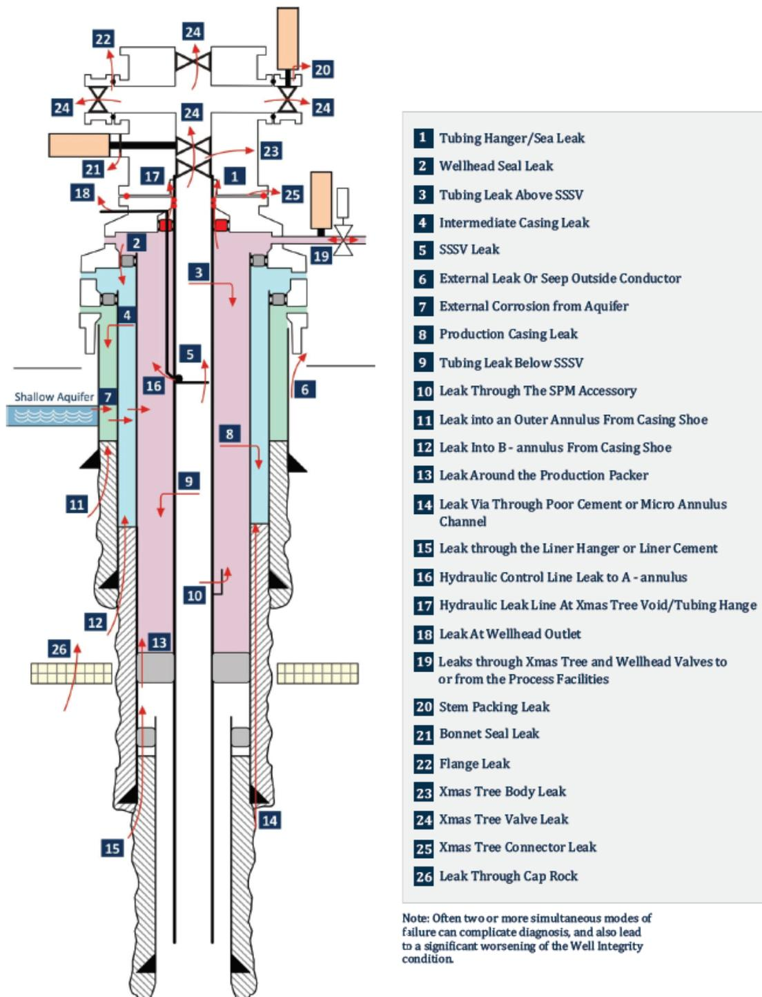
Figure: Well diagram showing some typical modes of well failure
