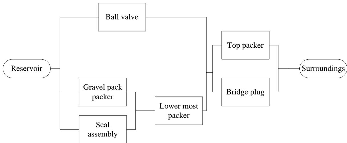
Figure 3: Barrier diagram for a temporary abandoned production well (from Holand, 1996).
