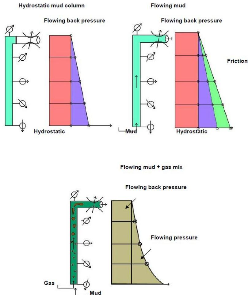
Figure 18: Illustration of the BHP in various situations in UBD (from Rigpass, 2012).
