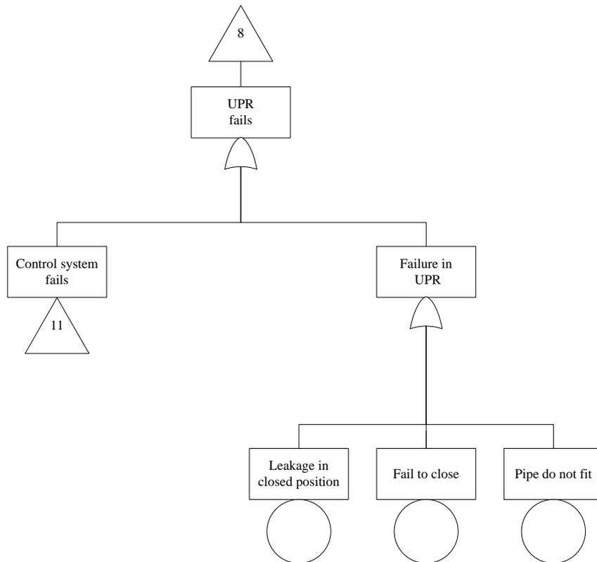
Figure 33: FT “Upper pipe ram fails”.
