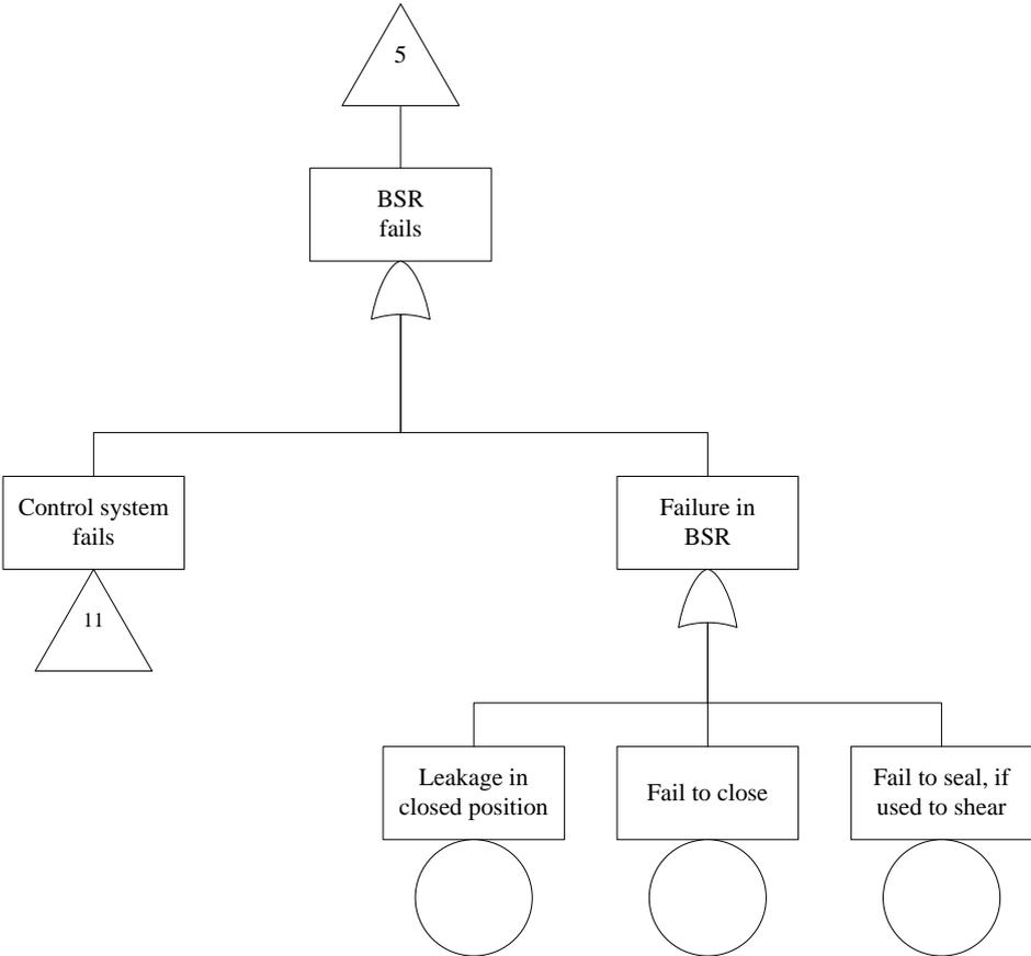
Figure 30: FT “Blind shear ram fails”.
