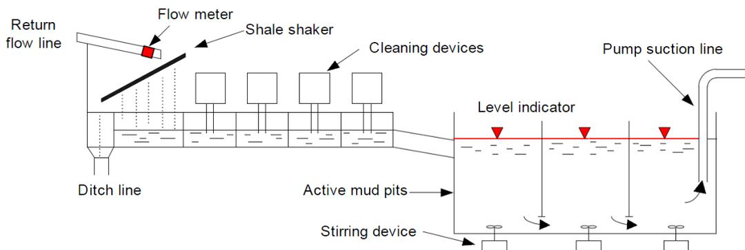
Figure 39: Surface metering of flow out compared to input flow, and of volume change in the pit (from Skalle, 2011).
