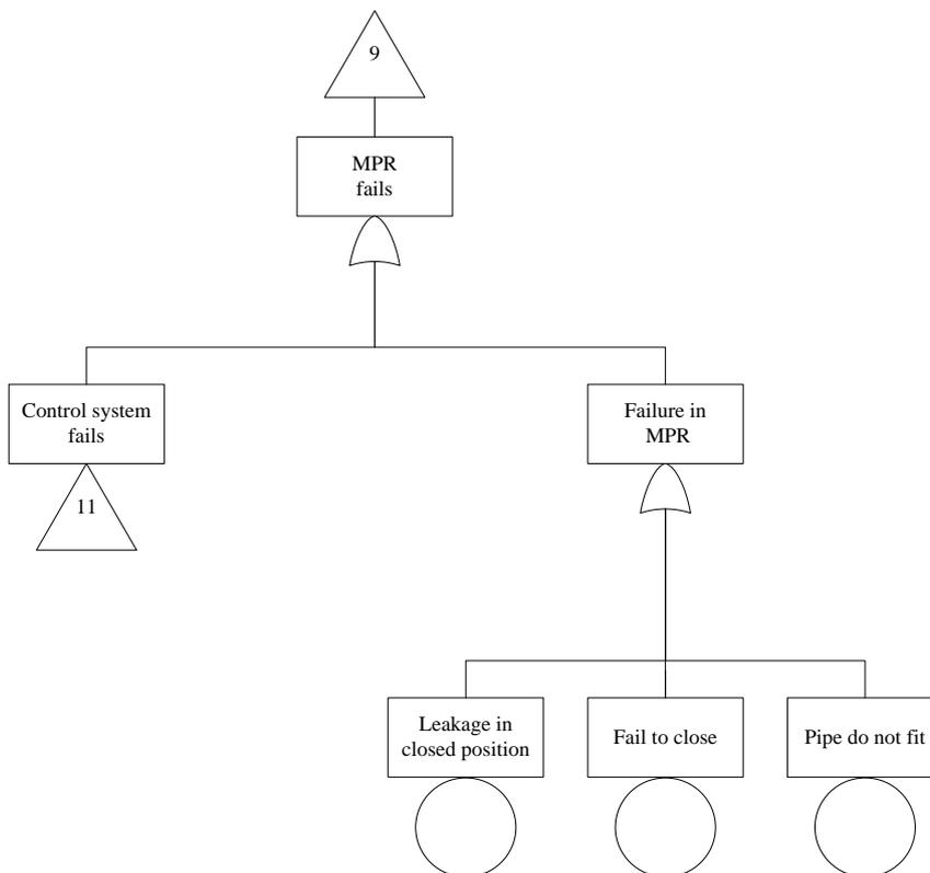
Figure 34: FT “Middle pipe ram fails”.
