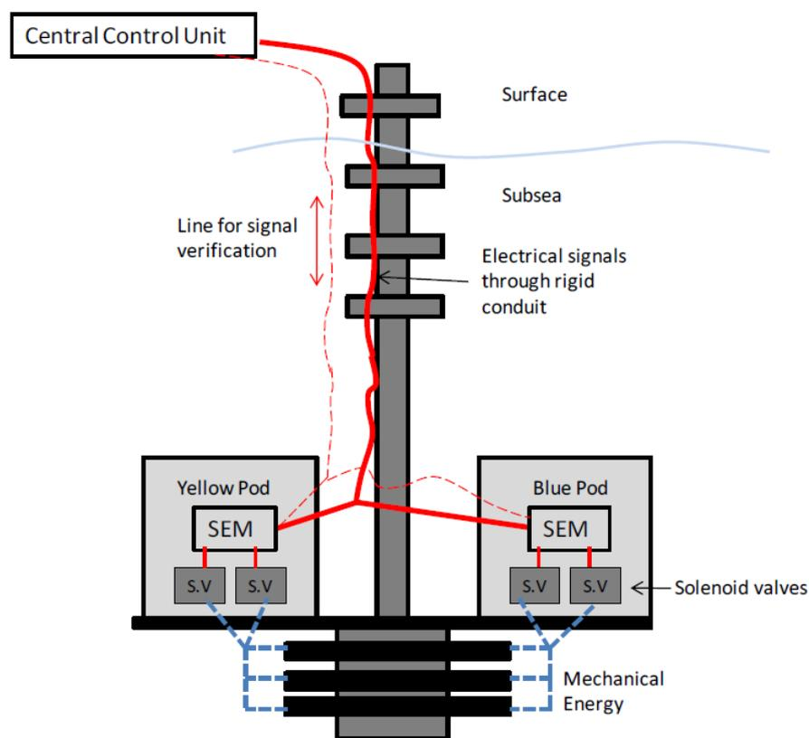
Figure 21: Basic principles of electro hydraulic/MUX control system (from Padøy, 2011).
