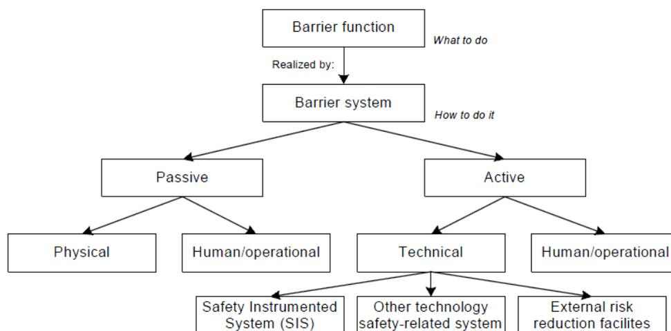
Figure 1: Classification of safety barriers (from Sklet, 2005).
