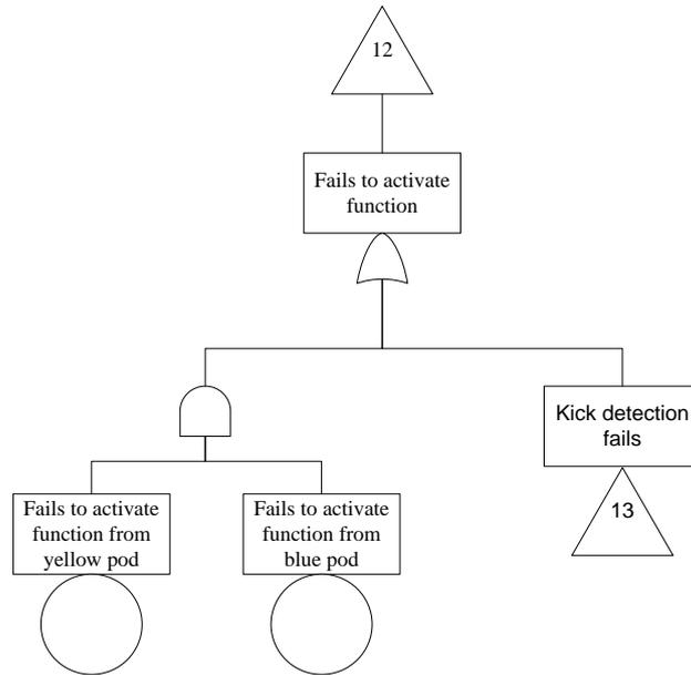
Figure 36: FT “Fails to activate function”.
