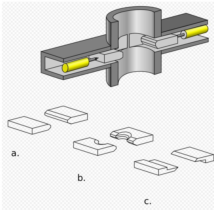
Figure 16: Illustration of the design for the blind ram (a), pipe ram (b), and the shear ram (c) (from Wikipedia, 2014).
