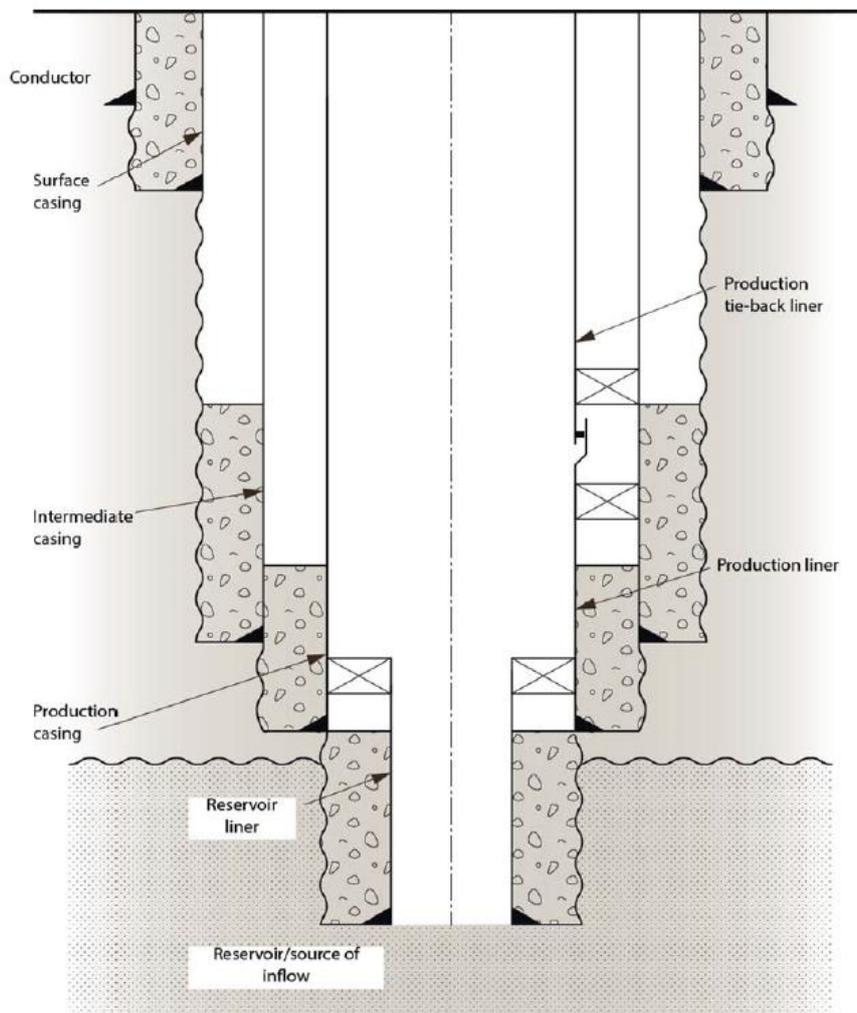
Figure 17: Casing illustration (from NORSOK D-010, 2013).
