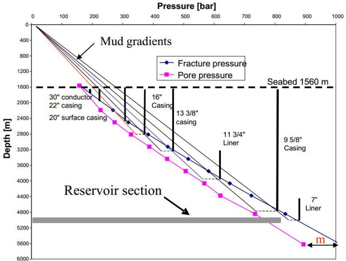
Figure 13: Typical casing program using a 18  $\frac{3}{4}$ " wellhead system (from TPG 4200, 2012).
