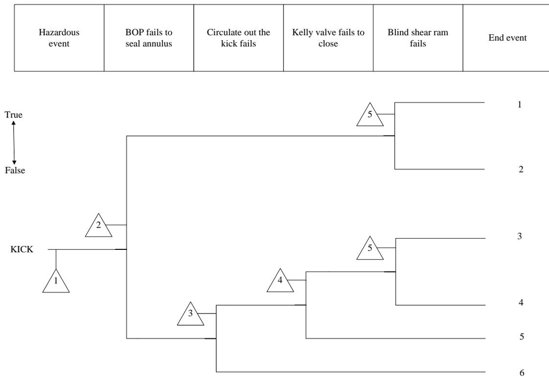
Figure 23: Simplified event tree. Drilling
