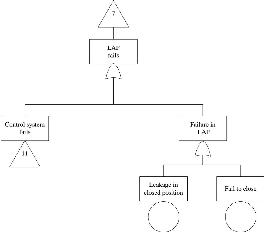
Figure 32: FT “Lower annular fails”.
