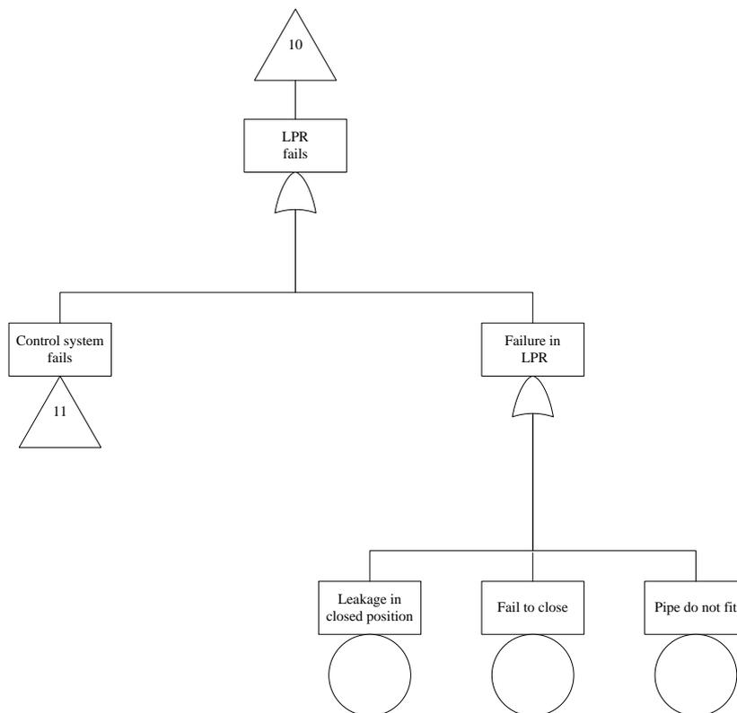
Figure 37: FT “Lower pipe ram fails”.
