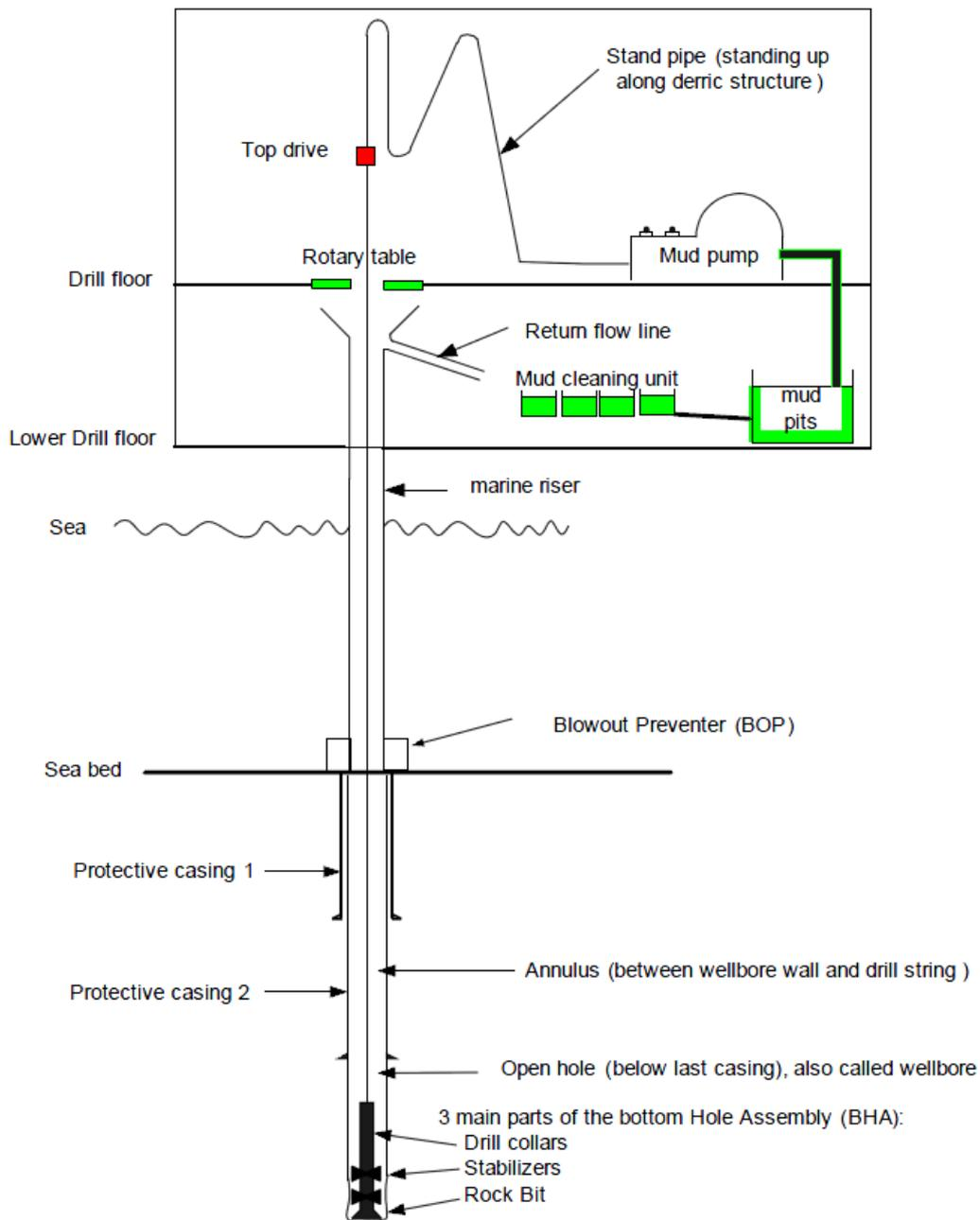
Figure 11: The drilling process (from Skalle, 2011).
