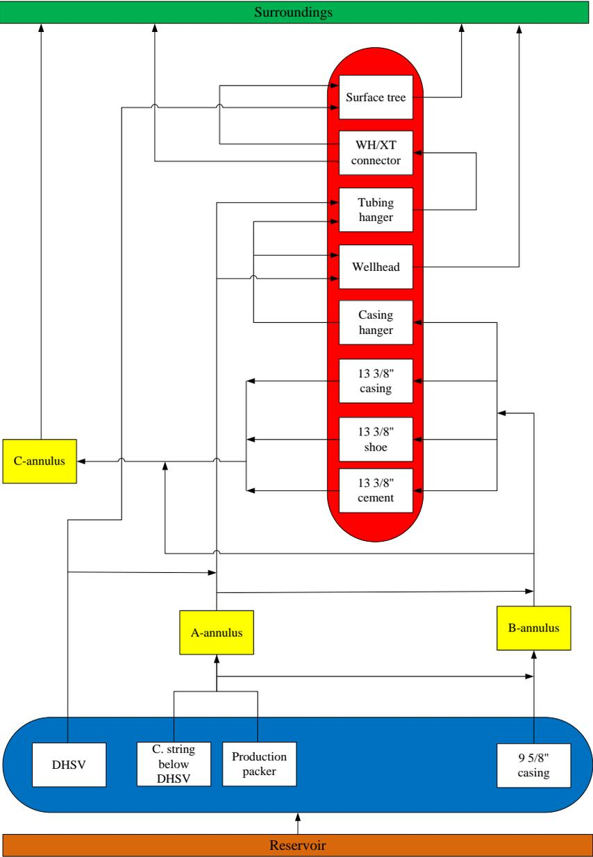
Figure 10: Well barrier diagram for a selected well.
