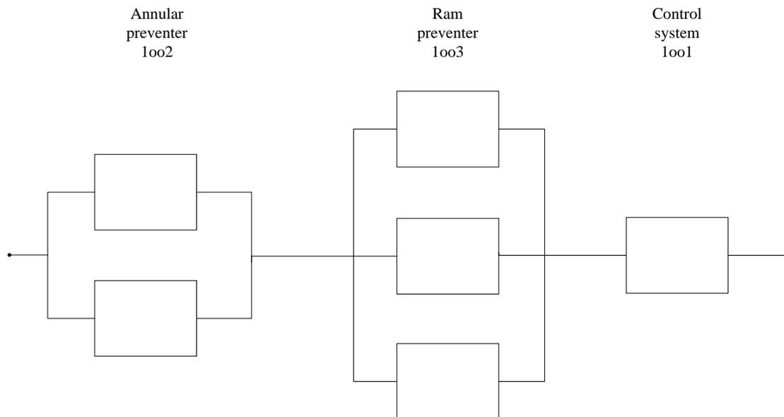
Figure 25: Block diagram of “BOP fails to seal annulus”.
