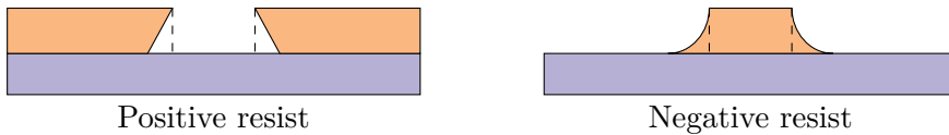
Figure 3.3.: Illustration of typical resist patterns affected by proximity effects. The dashed lines indicate the edges of the intended exposed areas.
