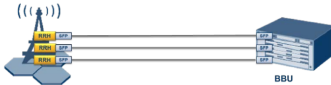
Figure 2.6: Point to point fiber [PMC15].
