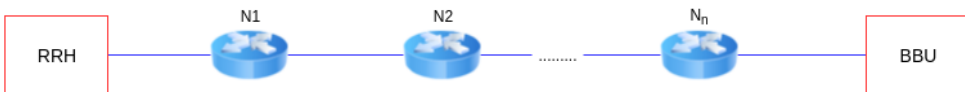
Figure 6.13: Mobile fronthaul network under study. The nodes can be either IHON node or Ethernet switch depending on the network under evaluation.
