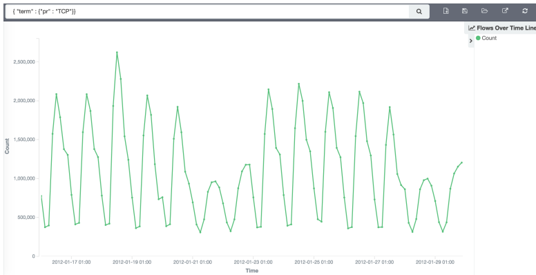
Figure 5.9: Flows over time diagram of two weeks' TCP traffic.
