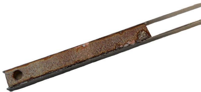
Figure 3.19: The design of the copper termination. The termination is soldered to three BSCCO HTSs.
