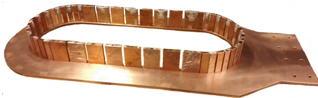
Figure 3.1: The bottom of the thermal interface with all the copper teeth mounted on the inner edge.
