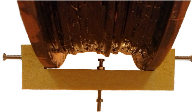
Figure 3.26: The mechanical holder for the Cernox sensor placed at bottom of the field winding.
