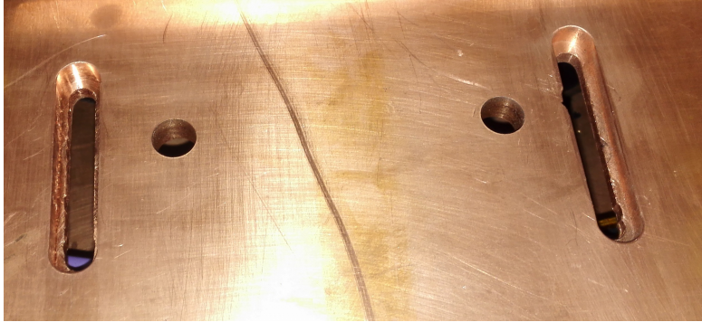
Figure 3.11: Grooves made in the thermal interface to attach the cooling pieces for the joints
