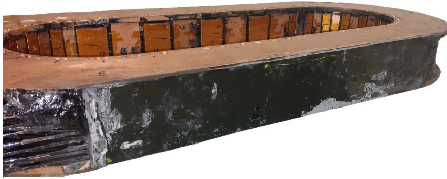
Figure 3.15: Surface after the mold was removed and epoxy spills were sanded away
