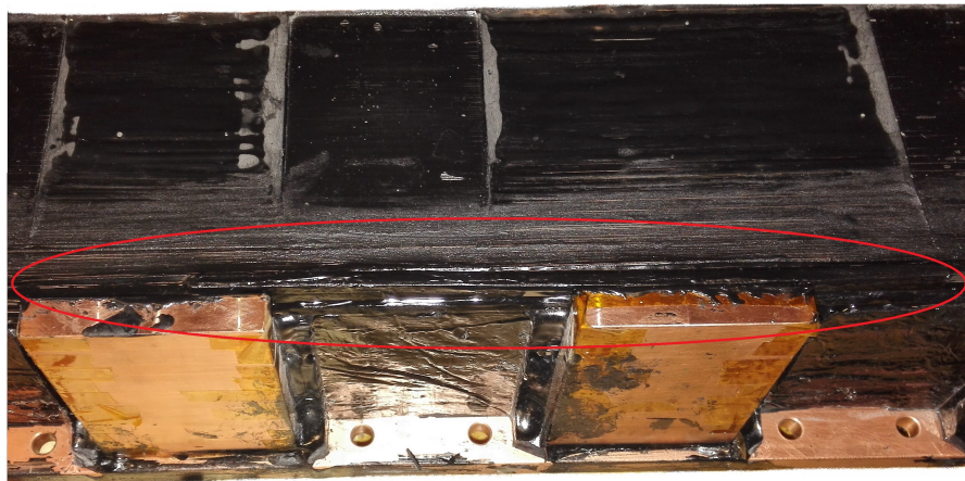
Figure 3.4: The pieces of superconductor that were placed between the tenth coil and the copper teeth.
