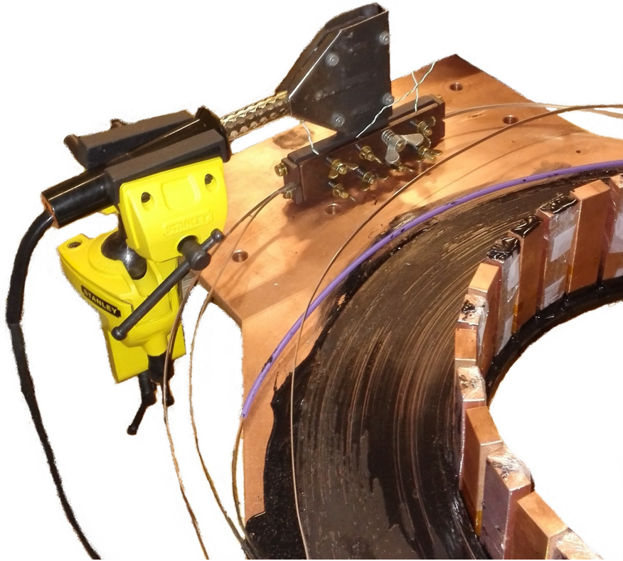
Figure 3.9: The first and second coil soldered together by the custom soldering tool. The soldering tool was held by a vise with a ball joint for mobility.
