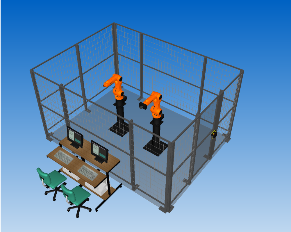
Figure 4.1: Graphic model of the KUKA Agilus robot cell at Department Of Production and Quality Engineering, NTNU
