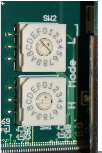
Figure 2 Hexadecimal switch orientation and software values
