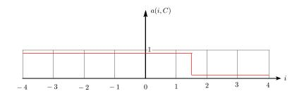
Figure 6: The function a(i, C) representing the LTS  $\beta$  scheme for a 9-point stencil with C = 1.5 and  $\beta = 0.1$
