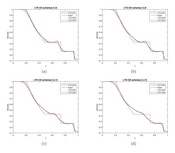
Figure 19: The Sod shock tube problem solved for Courant numbers 6, 9, 12 and 15 with different amounts of added numerical diffusion. The computational domain consists of 200 cells.
