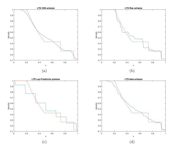
Figure 17: The Sod shock tube problem solved with the LTS CD6, the LTS Roe, the LTS Lax-Friedrichs and the LTS  $\beta$  schemes. The computational domain consists of 200 cells and  $\beta = \min(1, 30\Delta x/L)$ , and all schemes are computed with a Courant number C = 16.
