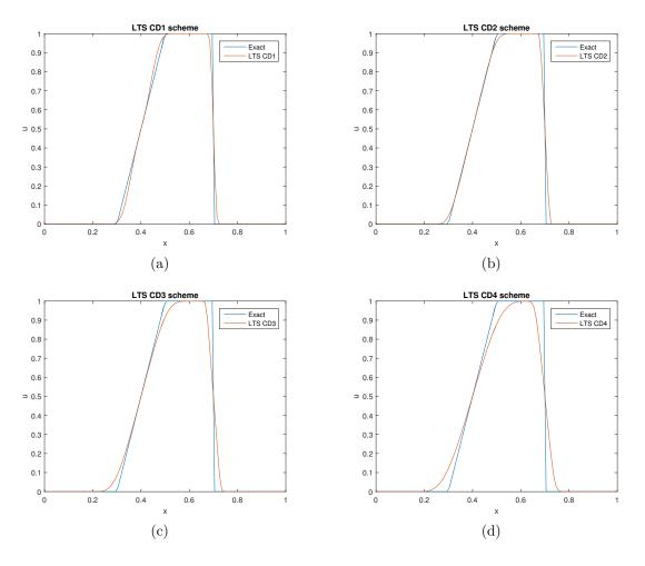
Figure 15: The 1 dimensional inviscid Burgers' equation acting on a square initial pulse, solved with LTS  $CD\hat{k}$  ( $\hat{k} \in 1, 2, 3, 4$ ) schemes with 100 cells after t = 0.2s. All schemes are computed with a Courant number C = 5.
