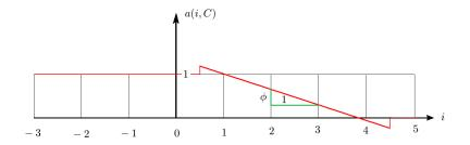
Figure 12: The function a(i, C) representing the LTS CD2- $\phi$  scheme for a 9-point stencil with C = 2.5.
