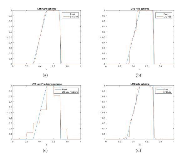
Figure 14: The 1 dimensional inviscid Burgers' equation acting on a square initial pulse, solved with various LTS schemes with 100 cells after t = 0.2s. For the LTS  $\beta$  scheme,  $\beta = 0.05$ . All cases are computed with a Courant number C = 5.
