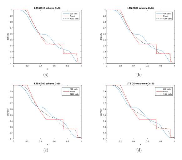
Figure 20: The Sod shock tube problem solved for Courant numbers 30, 60, 90 and 120 with a LTS  $CD\hat{k}$  scheme corresponding to the ratio  $\frac{k}{\hat{k}} = 3$ . The computational domains consist of both a course grid and a fine grid.
