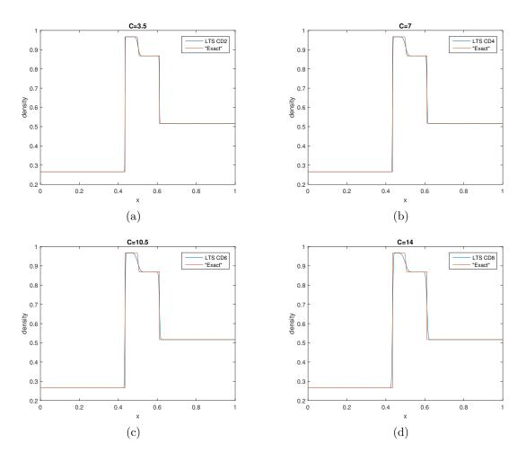
Figure 23: LeVeques test case solved for Courant numbers 3.5, 7, 10.5 and 14 with 2000 cells and an appropriate LTS  $CD\hat{k}$  scheme where  $\hat{k} = 2, 4, 6, 8$ , respectively.
