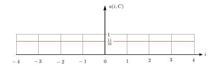
Figure 5: The function a(i, C) representing the LTS Lax-Friedrichs scheme for a 9-point stencil with C = 1.5
