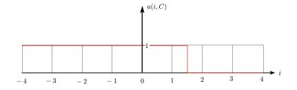
Figure 4: The function a(i, C) representing the LTS Roe scheme for a 9-point stencil with C = 1.5
