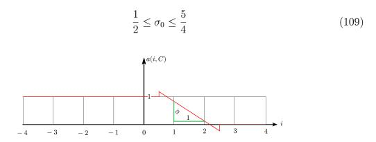
Figure 11: The function a(i, C) representing the LTS CD1- $\phi$  scheme for a 9-point stencil with C = 1.5.
