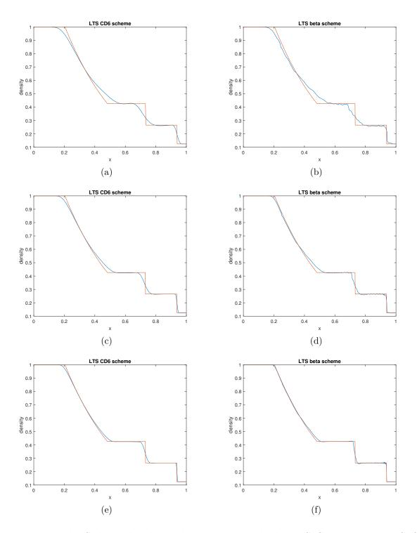
Figure 18: The Sod shock tube problem solved with the LTS CD6 and the LTS  $\beta$  schemes. The computational domain consists of 400, 800 and 1600 cells ranked from top to bottom.  $\beta = \min(1, 30\Delta x/L)$ , and all simulations are computed with a Courant number C = 16.
