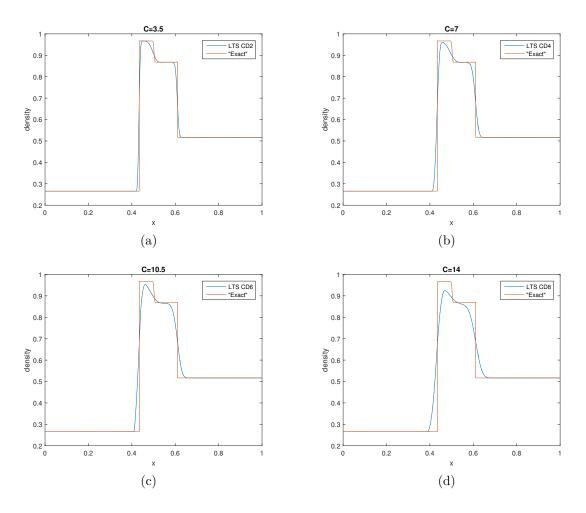
Figure 22: LeVeques test case solved for Courant numbers 3.5, 7, 10.5 and 14 with 400 cells and an appropriate LTS  $CD\hat{k}$  scheme where  $\hat{k} = 2, 4, 6, 8$ , respectively.
