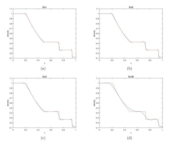
Figure 21: The Sod shock tube problem solved for Courant numbers 1, 2, 3 and 10 with the second order LTS  $CD\hat{k} - \phi - 2$  scheme corresponding to the ratio  $\frac{k}{\hat{k}} = 1$ . The computational domain consists of 200 cells.
