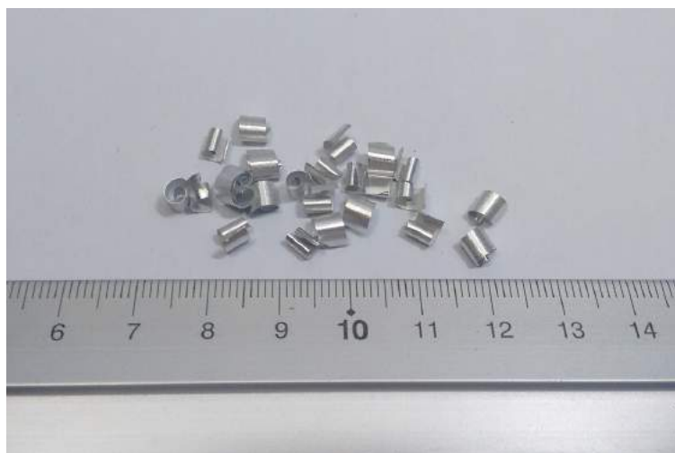
Figure 3.1: Machined granulates from DC cast billets.
