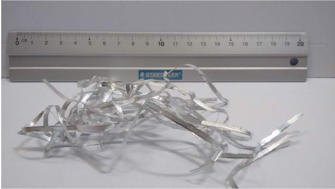
Figure 3.10: RS ribbons produced by melt spinning.
