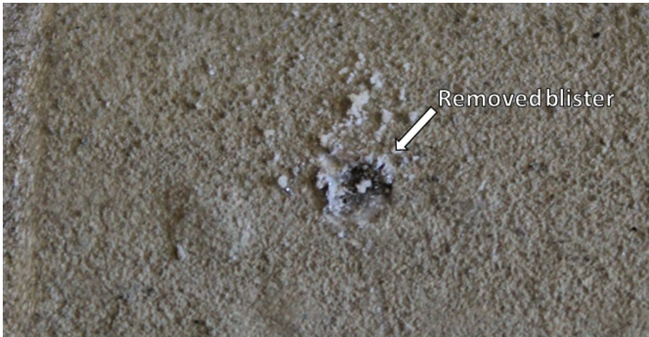
Figure 6.2: Photo of removed blistered on TSA exposed to seawater for 65 days 0 ° C internal temperature.
