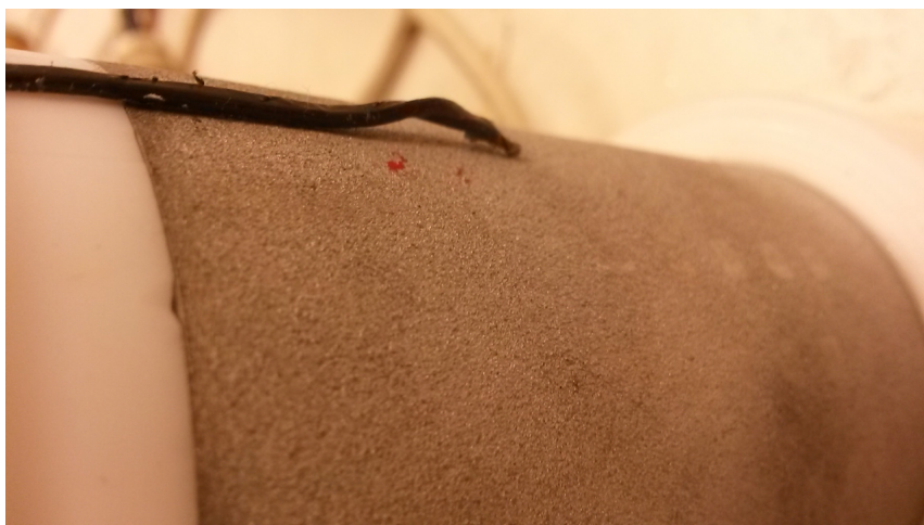
Figure 4.4: Mounting of Thermocouple on TSA surface before applying glue.
