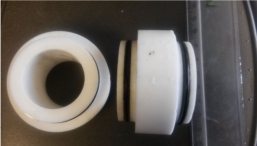
Figure 4.2: Isolation piece with O-ring gaskets.
