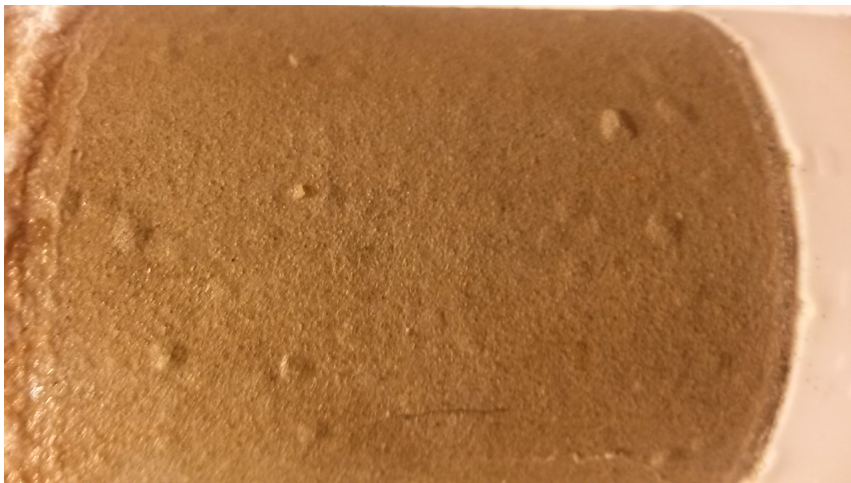
Figure 6.1: Photo of blisters in TSA exposed to seawater for 65 days with 90 ° C internal temperature.
