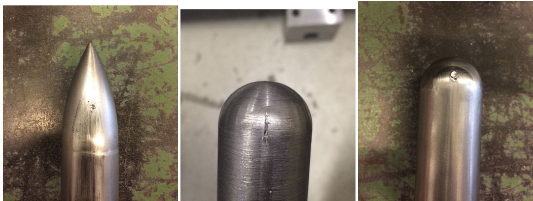
(a) Indenter 1 with damage (b) Indenter 2 with damage (c) Indenter 3 with damage
