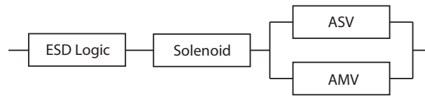
Figure D.1: Example of a block diagram for both E-ASV and H-ASV
