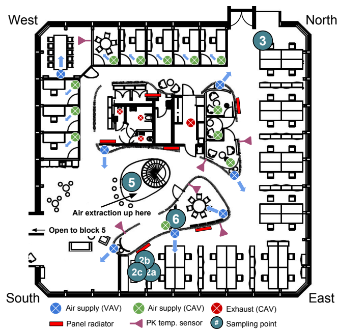
Figure A.1: Location of sampling points for tracer gas measurement on March 9, 2016 - second set
