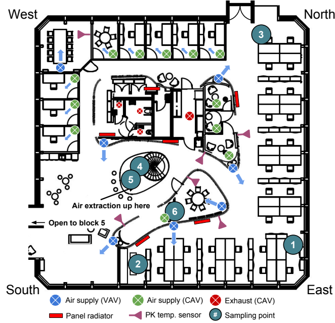
Figure 3.2: Location of sampling points for tracer gas measurement on March 9, 2016 - first set
