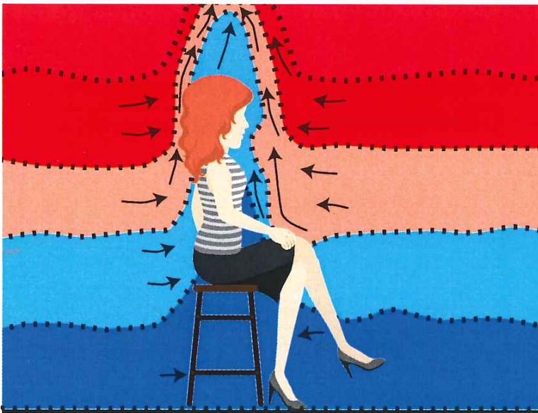
Figure 2.4: Local convection forces provide better air quality in the breathing zone (Ingebrigtsen, 2015)
