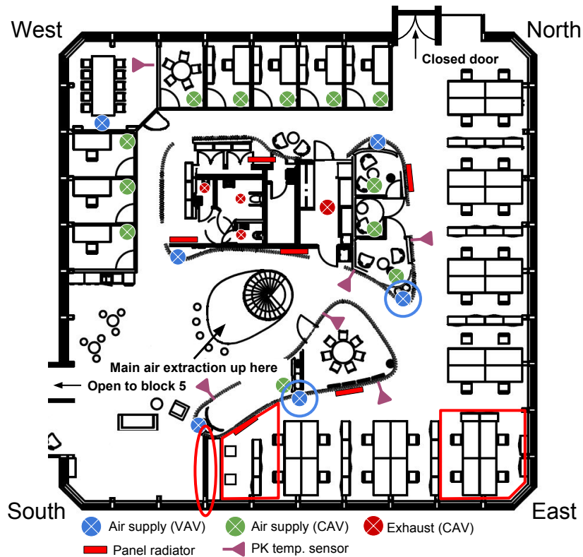
Figure 1.1: Floor plan of second floor of building four. The diffusers in question are highlighted by blue circles. The zones suspected of having stagnant zones are highlighted in red. The red oval indicate a separating wall. Figure is based on illustration by Søgnen (2015)
