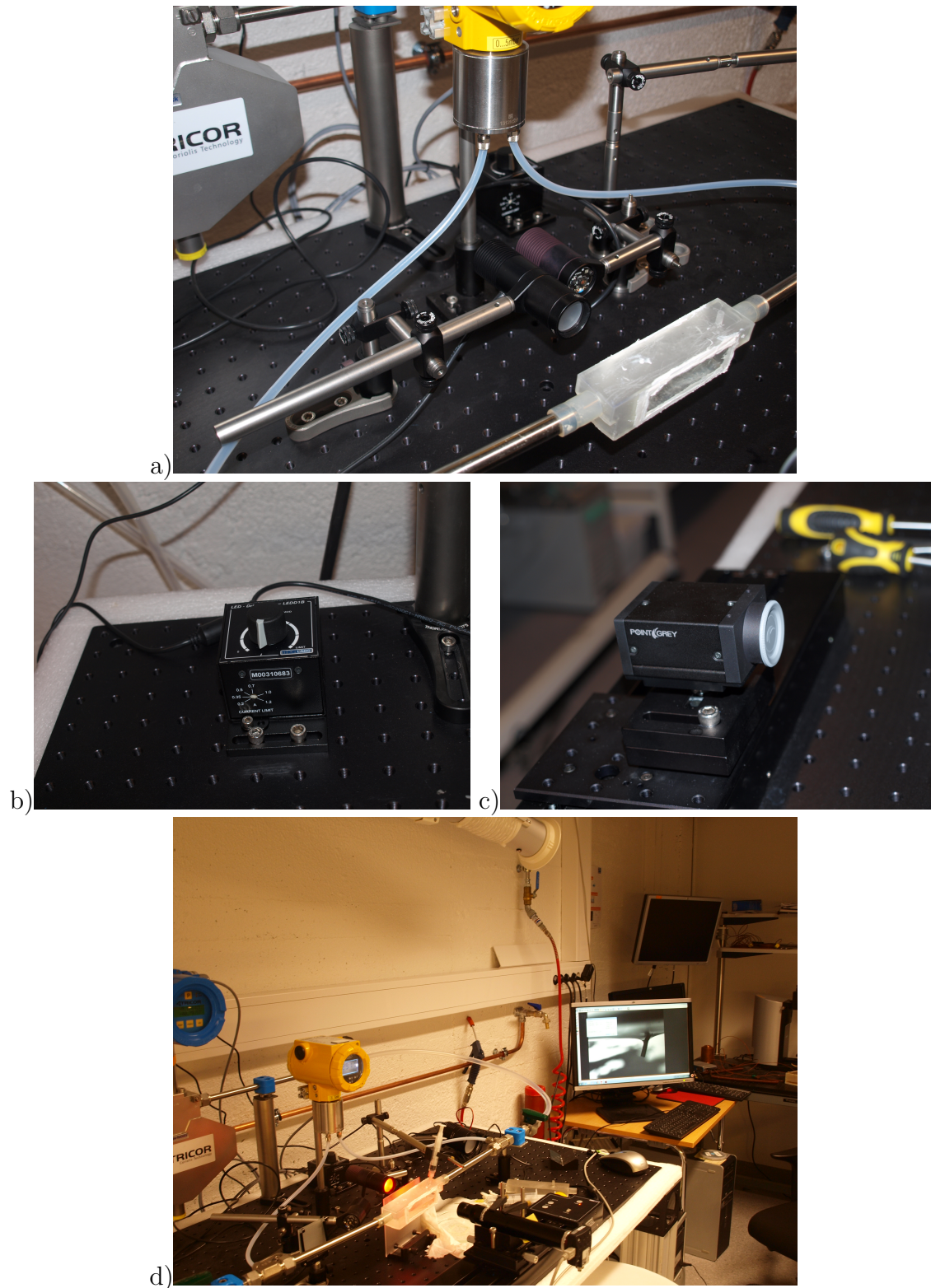
Figure 4.9: a) LEDs stands. b) T-cube LED driver. c) Grasshopper camera. d) Computer.
