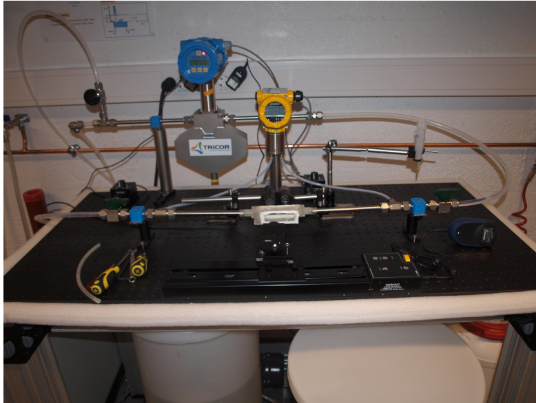
Figure 5.3: Close loop of the facility with measuring instrumentation.
