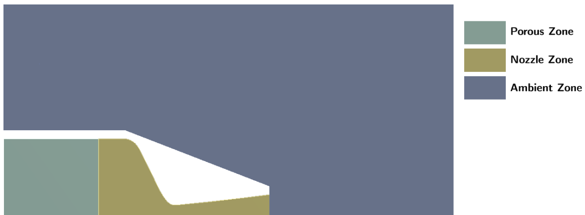
Figure 4.1. Geometry setup in Fluent split into the porous, nozzle and ambient zones.
