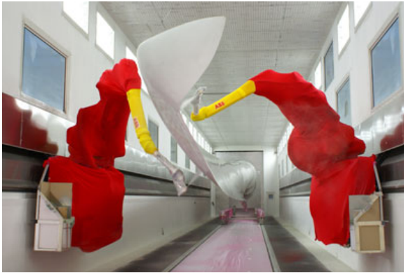
Figure 2.10: Coating rotor blades (ABB.com, 2012).
