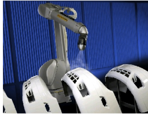
Figure 2.11: Coating of car parts (Fanucrobotics.com, 2012).
