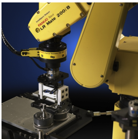
Figure 2.16: Fanuc during assembly operation (Fanurobotics.com, 2012).
