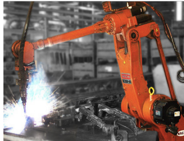
Figure 2.13: Arc welding operation (Nachi-robotics.com, 2012).
