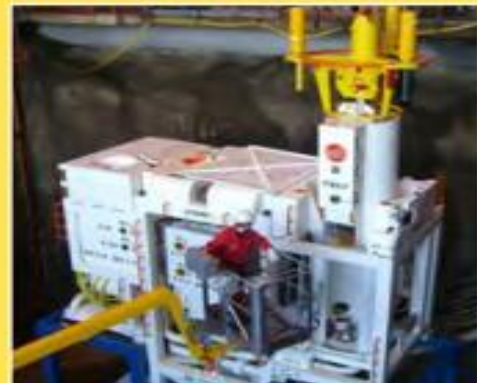
Fig.8: OneSubsea's Testing of the Albacore Raw Seawater Injection System during SIT of Pump and Filtration System
