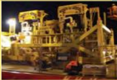
Fig. 1: Aker Solutions' LiquidBooster™ Subsea Raw Seawater Injection System (Photo: System for Statoil Tyrihans Subsea Raw Water Injection Project)
