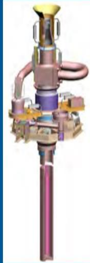
Fig. 9: FMC Technologies Vertical Access Caisson with ESP Boosting (Gas/Liquid Separation & Boosting System Diagram)
