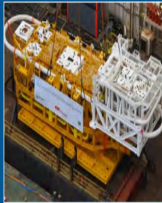
Fig. 12: FMC Technologies 3-Phase Separation System with Produced WI Using In-Line Separation Technology for the Marlim Project
