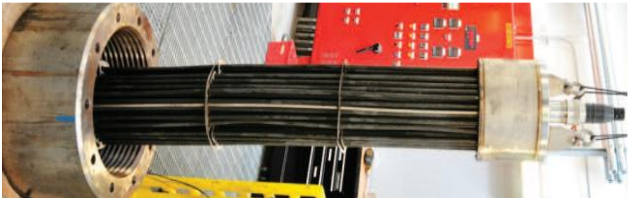
Figure 5.21 Subsea Heater, 5000V, 3500m depth
