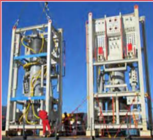
Fig. 2: OneSubsea Multiphase Compressor Units for Gullfaks Field
