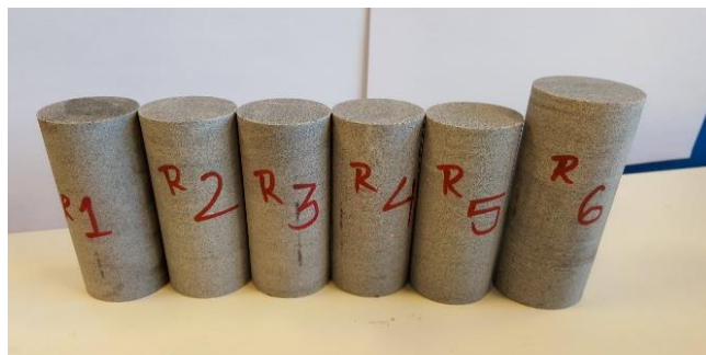
Figure 2-2: Cylindrical shape specimen for Uniaxial Compression Test
