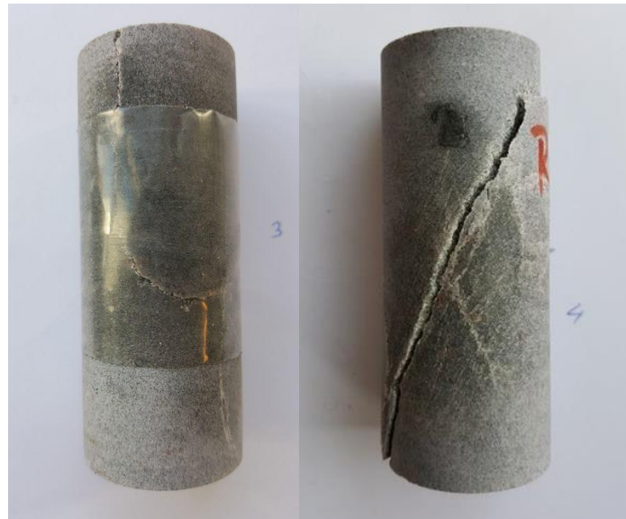
Figure 4-4: Core sample after UCS test. Left is sample no. 3 and right is sample no. 4
