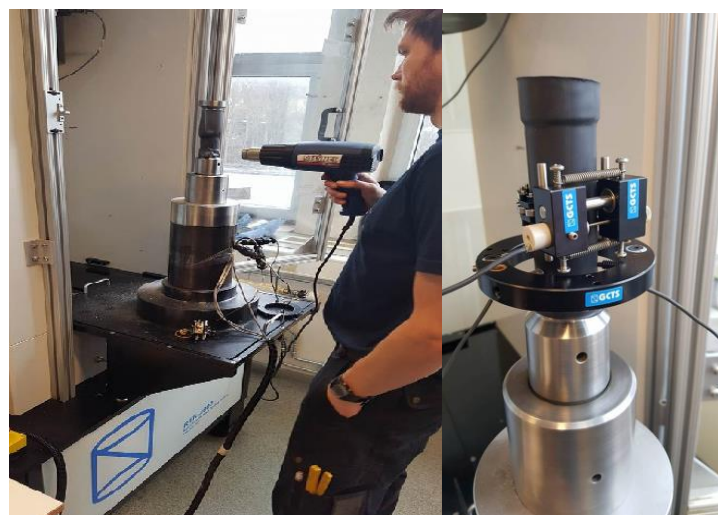
Figure 4-3: Sample preparation for UCS test (IGB Laboratory at NTNU)
