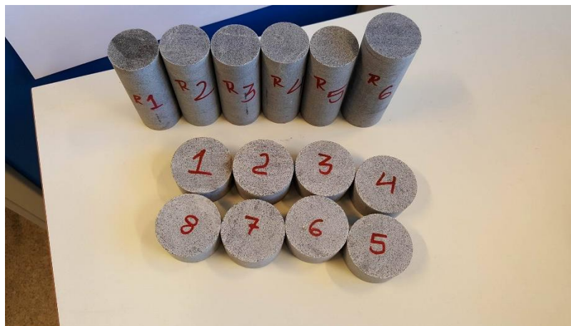
Figure 4-2: Samples prepare for UCS test (above) and Brazilian test (below)
