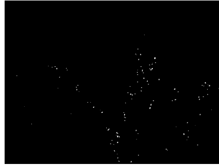
(b) Multiple channels observed in reference image with AV = 60 kV. v_{BD} = 2.5 mm/ \mu s.
