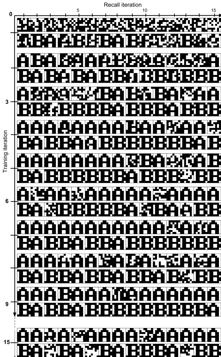
Figure 4.2: Displaying the neural network recall for the training inputs after each training iteration. Note that the origin is now in the upper left corner, time flowing downward along the y-axis for each training iteration, with the first axis denoting the model recall iteration. Note that for each training iteration, there are two rows of recalled output, displayed for two corresponding inputs, namely the two inputs of the current training subset. In this figure, these are the patterns 'A', and 'B', for the upper and lower rows, respectively. The model configuration is using synchronous CA3-updating, turnover only after the set is learnt, and a DG-weighting of 25.
