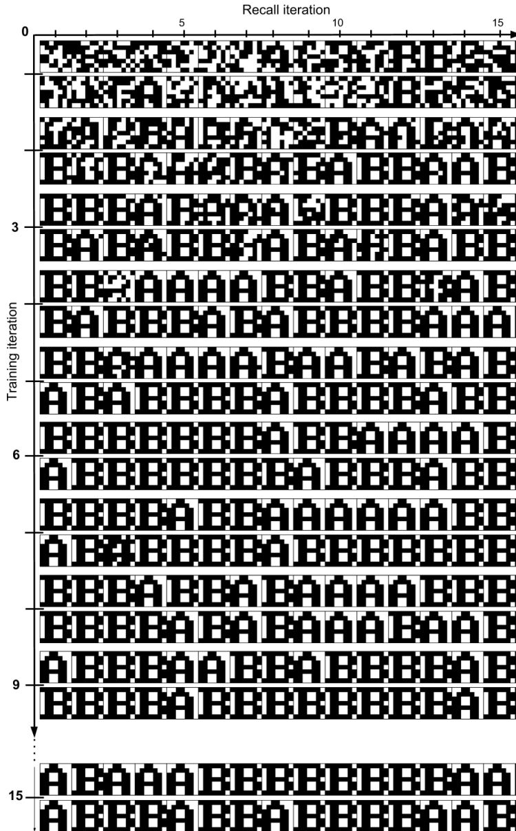
Figure 4.4: Showing the recalled outputs for the training inputs of the subset, after each subset training iteration, similar to in figure 4.2. However, the model configuration used here is asynchronous CA3 updating, neuronal turnover between every learnt set, a DG-weighting of 1, and \tau = 0.50 .
