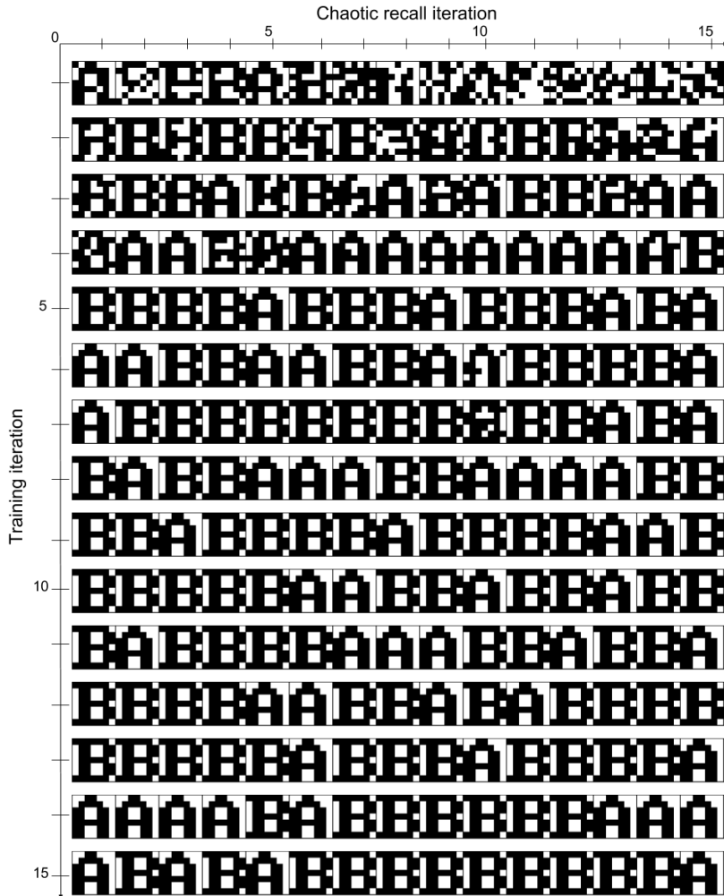
Figure 4.5: Displaying the chaotically recalled patterns for the same model configuration and results as displayed in figure 4.4 (asynchronous CA3-updating, a DG-weighting of 1, \tau = 0.50 , turnover between learnt sets). Note that spurious patterns diminishes very quickly, and only learnt patterns are chaotically recalled after very few iterations. This configuration seems to be capable of one-shot learning.
