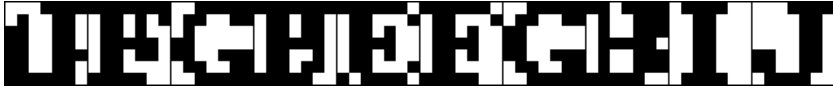
Figure 4.30: Displaying the recalled output of the neocortical network after training on the original associative training pattern subsets , 15 iterations per subset. Note that the first 3 out of 5 subset outputs are completely distorted, and do not resemble the desired output at all.
