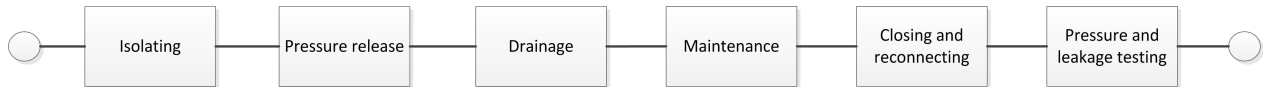
Figure 6.1: RBD of the operating process regarding maintenance procedure on pressurized hydrocarbon processing equipment
