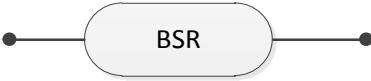
Figure 6.6 Available barriers for the DWH Stack with no objects going through the BOP
