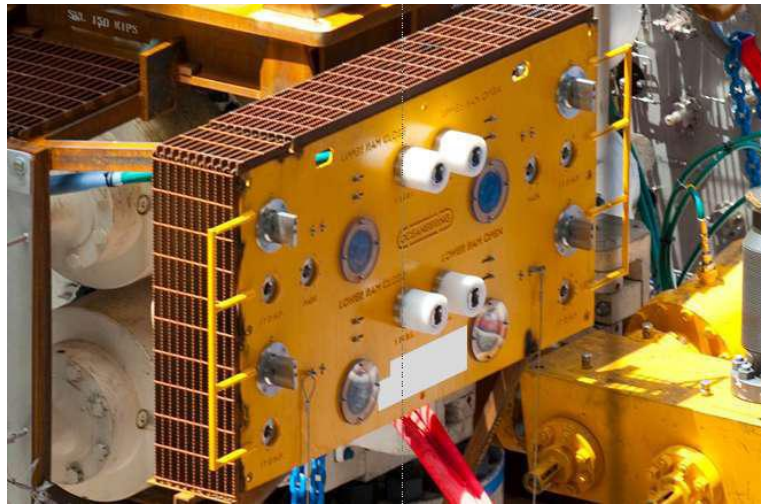
Figure 4.6 ROV Activation Panel (Potter, 2010a)
