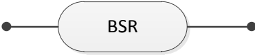
Figure 6.8 Available barriers for the classical stack with no objects going through the BOP
