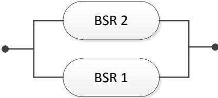
Figure 6.7 Available barriers for the modern stack with no objects going through the BOP
