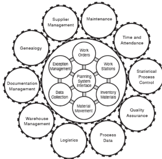
Figure 33 Core and support functions of MES
