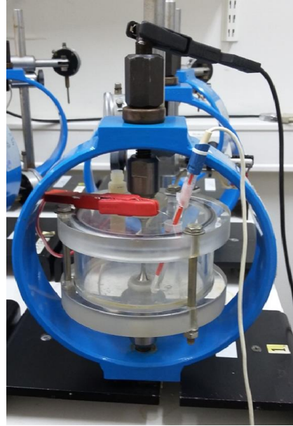
Figure 3.11: Picture of experimental setup for the stepwise loading in Cortest proof rings - hydrogen exposed sample.
