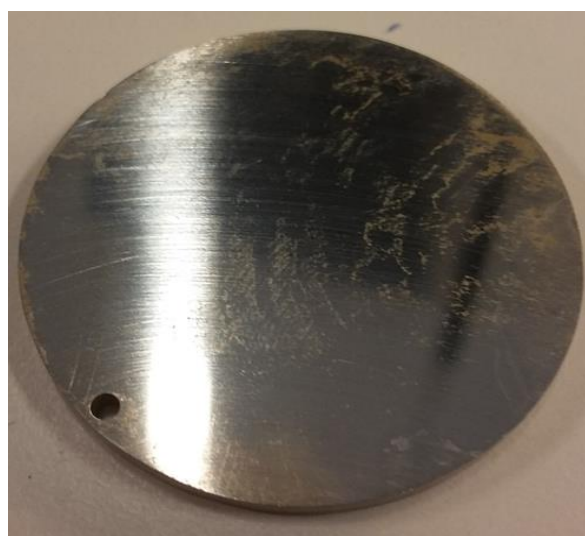
Figure 4.57: Sample F1010-2 after the modified ASTM G48 test showing a red/brown deposit on the surface.
