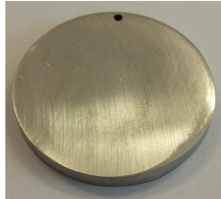
Figure 3.6: Picture of the sample used in OM, EDS, hardness test and modified ASTM G48 test.
