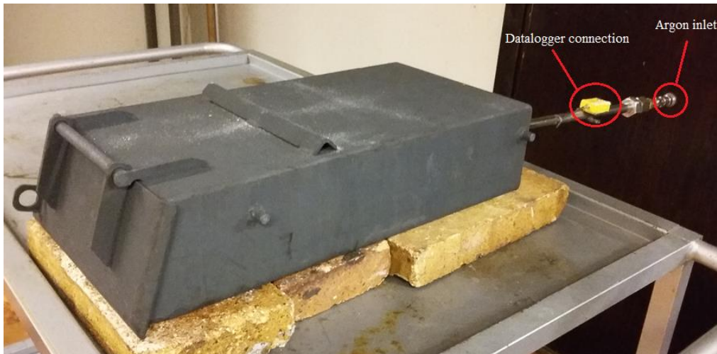
Figure 3.7: Box used during heat treatment to maintain an argon atmosphere.
