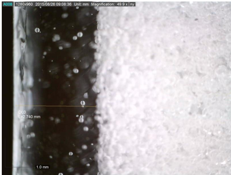
Figure 19. 50x magnification light microscopy image from wall of a used crucible, clearly showing the bubble free (BF) layer to the left and bubble containing (BC) layer to the right.
