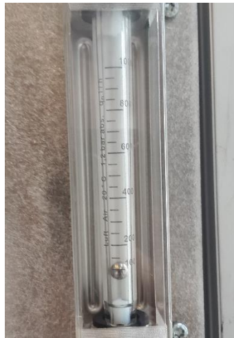
Figure 23. Argon flow through the furnace.
