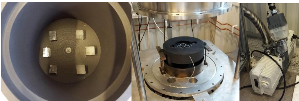
Figure 22. Left: Samples placed in the graphite crucible, middle: Open furnace, heater seen inside the graphite, right: The oil fume filter on top of the vacuum pump.
