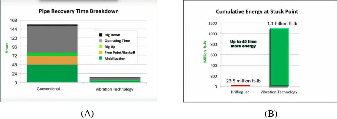
**Figure A.2** Charts highlighting the benefits of resonant vibration for releasing stuck pipe compared to conventional method with regards to recovery time and actual energy transferred to the stuck point (Layne, 2015).
