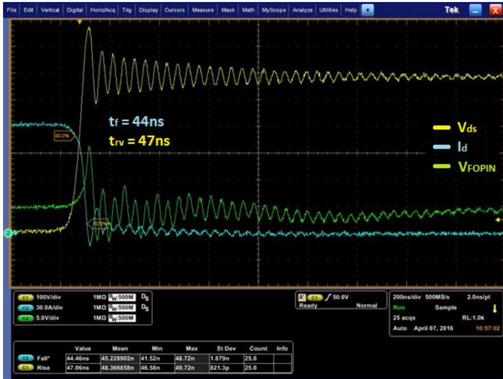
Figure 7.17: Hard-switching DUT turn off at 600 V 120 A
