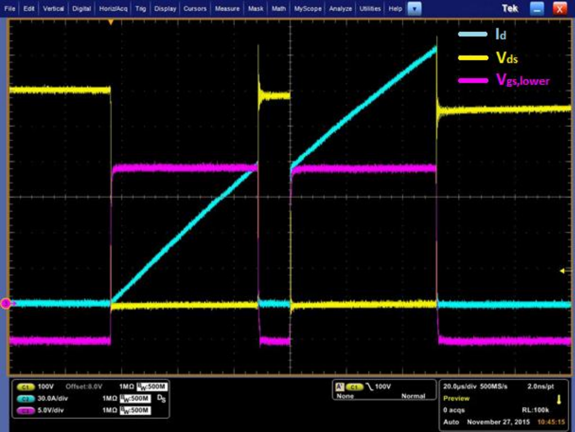
Figure 5.16: 600 V 120 A double-pulse test with L = 250 \mu\text{H}
