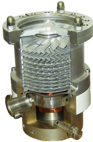
Figure 3.19: A cut through turbo-molecular pump. The gas molecules enters at the top of the turbopump, and gain momentum through the stack of rotating blades. In the bottom left a roughing pump is connected to the flange and the gas is pumped out of the system. Figure taken from Ref.[60]
