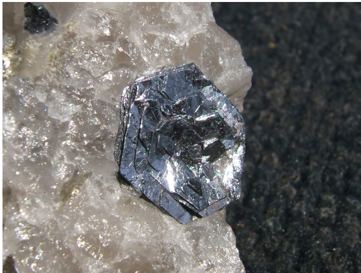
Figure 2.1: MoS 2 crystal. The crystal has large crystal domains and forms in a layered structure. Picture taken from Ref.[17].
