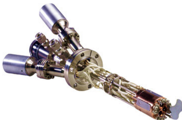
Figure 4.3: Mini e-beam evaporator. The evaporator is mounted on the outside of the vacuum directed towards the sample. Water cooling goes through the pipes, and there is the possibility to have shutter in order to deposit multiple materials. Figure taken from Ref.[61].
