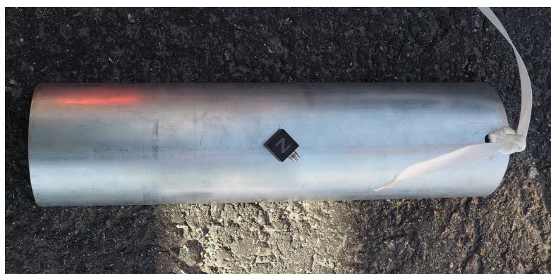
Figure 5.6: Accelerometer mounted to steel section
