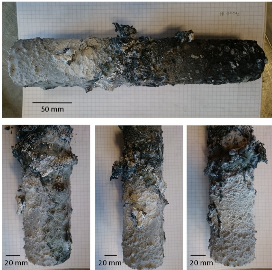
Figure 4.24: Visual inspection of sample V4 in different views, after exposure to silicon and slag in the induction furnace.
