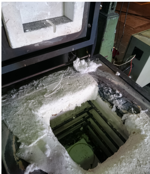
Figure 3.5: Image of the Entech electric resistance heated furnace used in the experiments.
