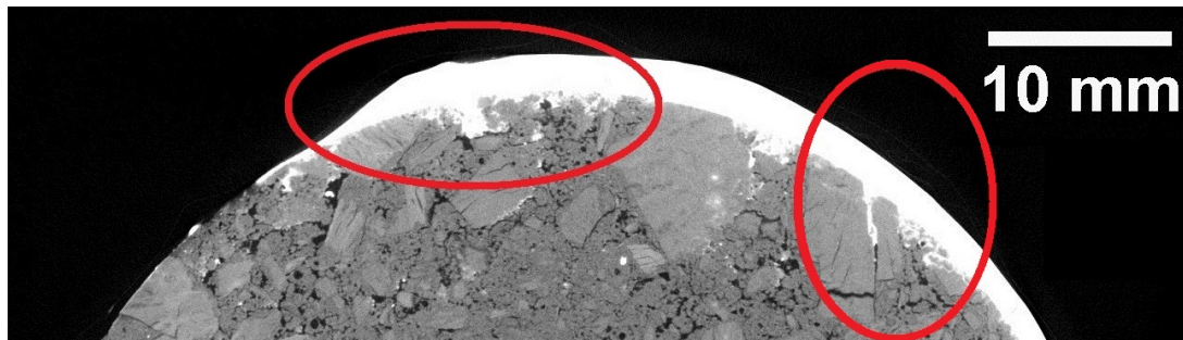
Figure 4.60: Intrusion in anthracite grain and binder phase, 5.2 cm into sample V8.
