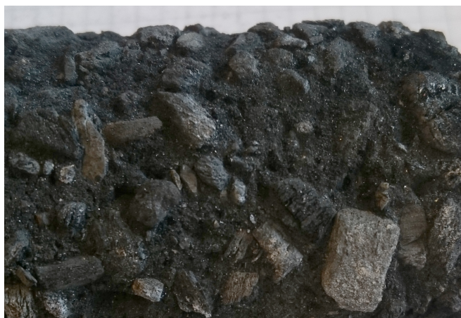
Figure 2.16: Example of carbon lining erosion, where the binder phase has eroded while the larger anthracite grains remain.
