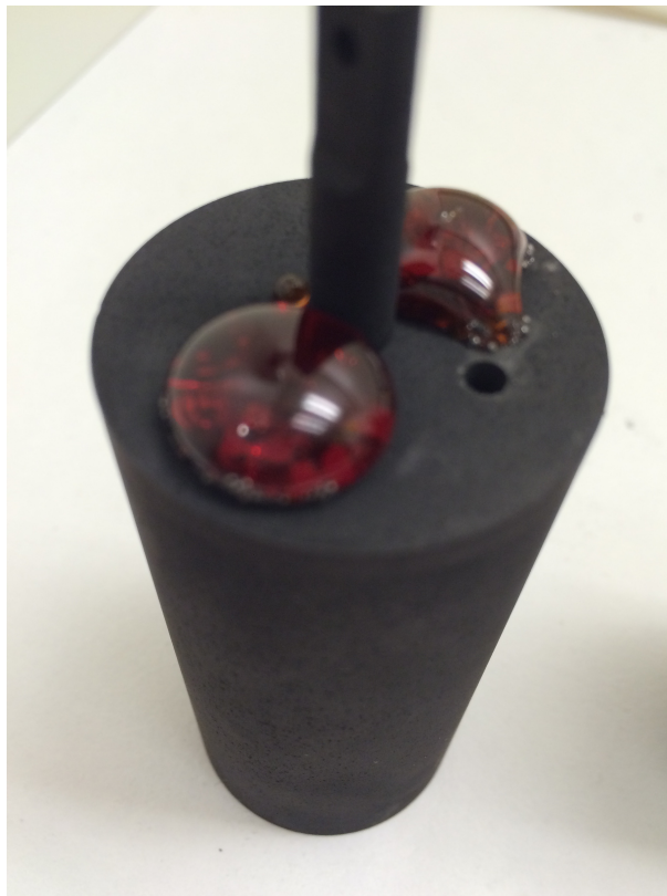
Figure 4.14: Picture of the crucible after Experiment L2. It was found slag on the top of the lid.
