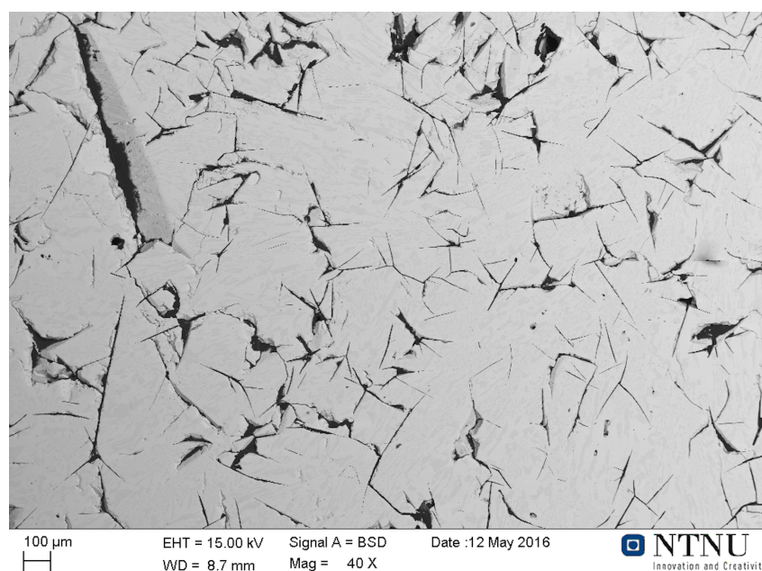
Figure 4.3: SEM image from Sample Q1. Metal phase.
