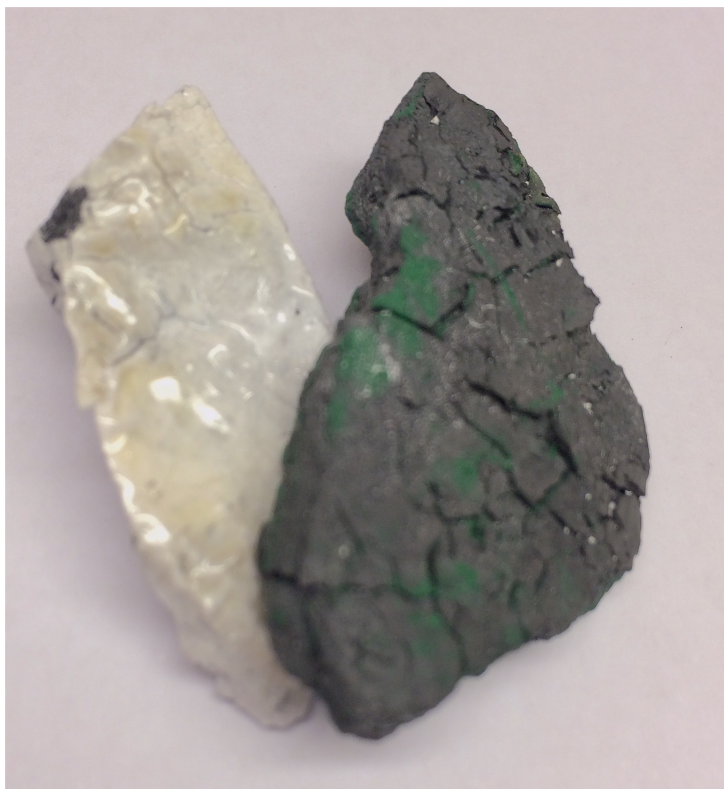
Figure 4.24: Picture of Sample L3. Quartz and Comilog ore piece after heating to 1350 °C.
