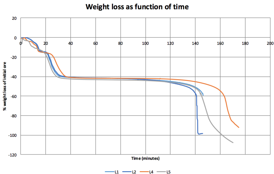
Figure 4.21: Weight loss graphs for experiments at high temperature with limestone as function of time.
