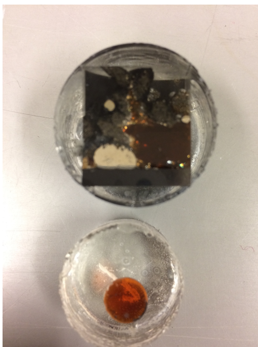
Figure 4.12: The Samples prepared for the EPMA. The slag from the top of the lid is also prepared as shown in this picture.
