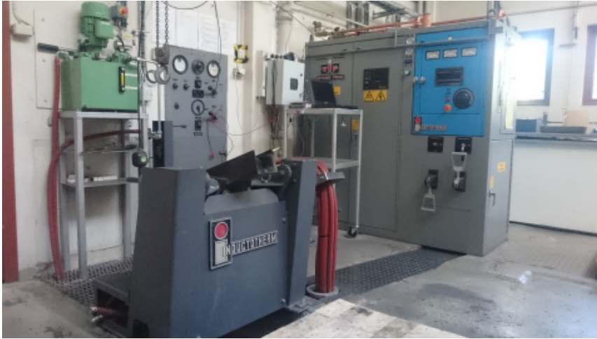
Figure 4.3: IF75 furnace used in the melting experiments
