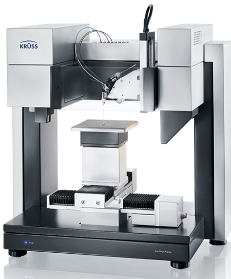
Figure 3.8: The DSA100 from Krüss used for contact angle measurements.
