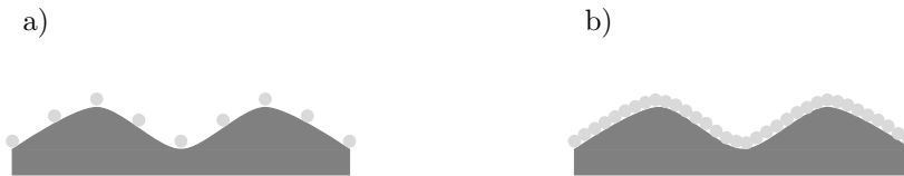
Figure 5.2: Illustration of surface structures obtained by deposition of different amounts of NPs. a) NPs spread out on the surface and b) NPs deposited in an even layer. The nanoroughness shown in a) is larger than that in b). The microroughness of the underlying substrate is identical in the two illustrations.
