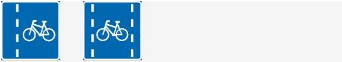
Figure 2-7 – Sign indicating that there is a cycle lane on one or both sides of the mixed road.
