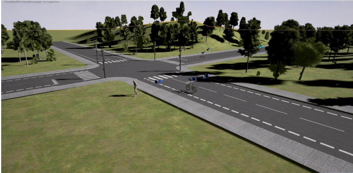
Figure 4-10 – The finished 3D environment for the test scenarios. This includes working traffic lights, surrounding terrain with vegetation 1 , and some other features like lighting and a skybox that is part of Unreal Engine 4 already.
