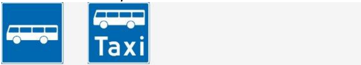
Figure 2-8 – Sign indicating public transport lanes.
