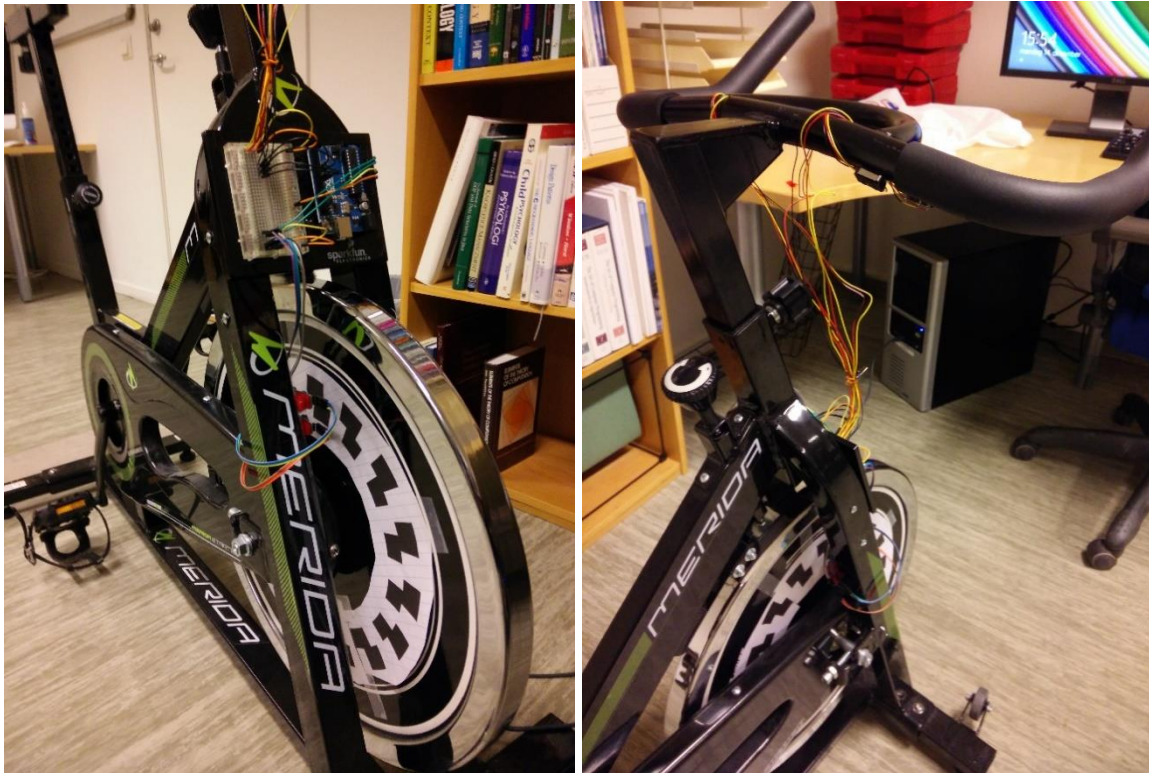
Figure 2-2 – The controller. The left picture shows the Arduino and the breadboard that connects all the wires. One can also see the sensors that measures the speed of the front wheel. The right picture shows the handlebar. You can see one of the buttons on the right side. This picture got two buttons on each side, but one can add as many as one needs.
