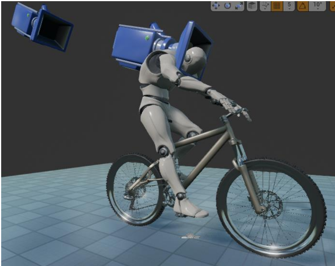
Figure 2-1 – The virtual cyclist model. The blue cameras are used to get a first- or third-person view when cycling.
