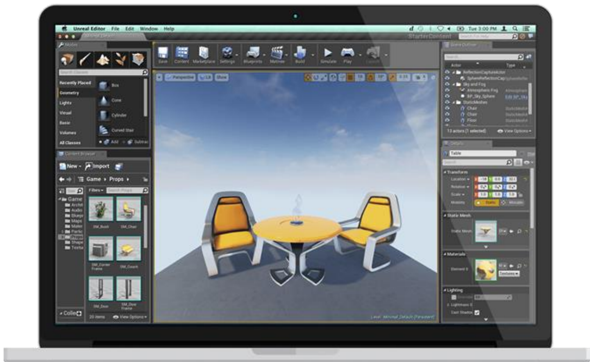
Figure 2-5 – The standard Unreal Engine 4 Editor window. On the left one can see tools for editing and adding objects to the 3D world. In the middle is the 3D environment, this can be interacted with, even used to play a game. On the right is the property windows for a selected object. This allows manipulation of an object in several ways.
