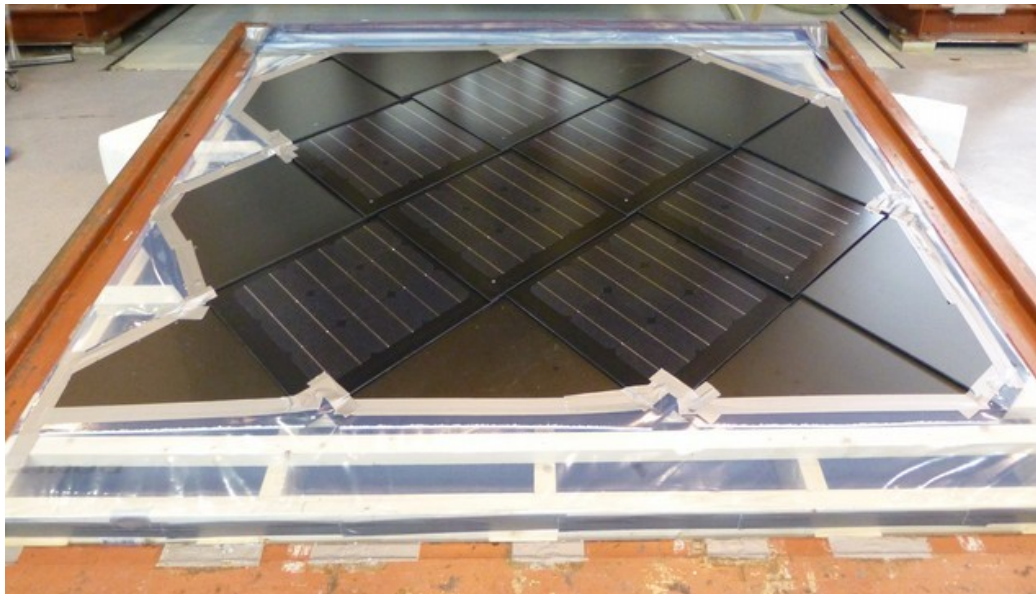
Figure 5: GS Integra Line SP, configuration B, with a greater number of PV modules. The corners where four PV modules meet are particularly important.
