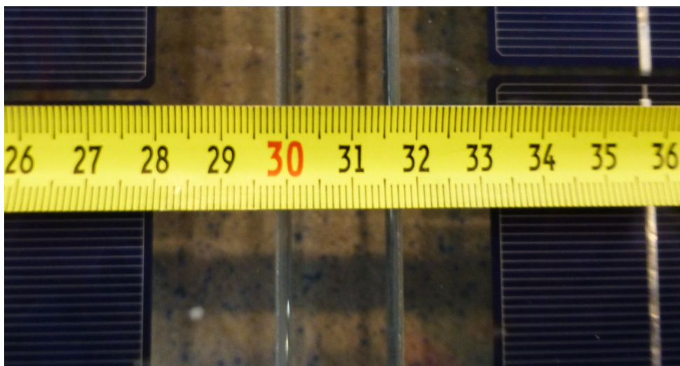
Figure 3: The gap between Solitek PV Modules using the supplied clamp fastening system.
