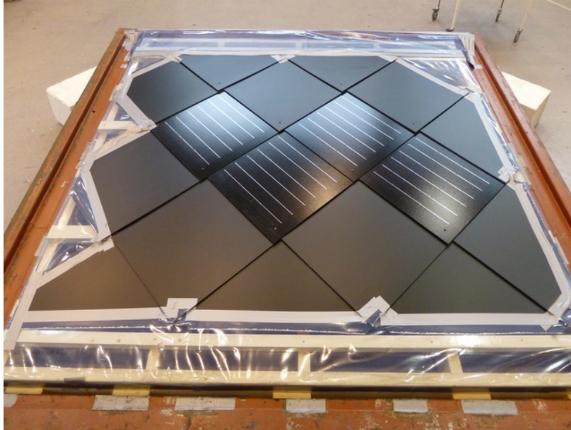
Figure 4: GS Integra Line SP, configuration A, mounted on a substrate frame and ready to be inserted in the RAWI box.
