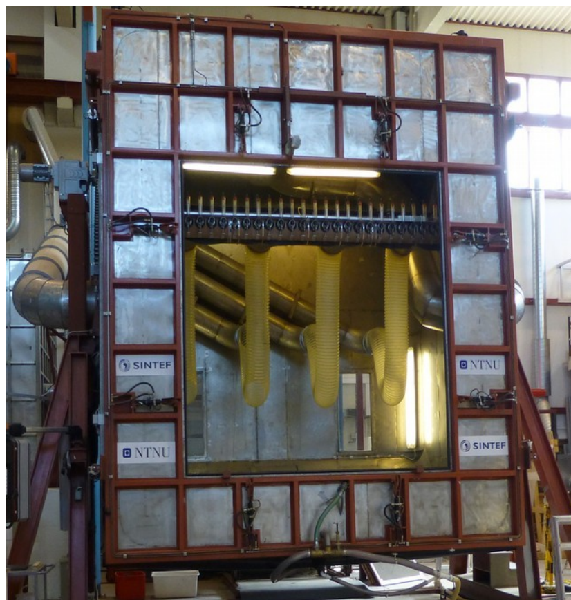
Figure 1: The RAWI box in the NTNU and SINTEF Building and Infrastructure Laboratory.
